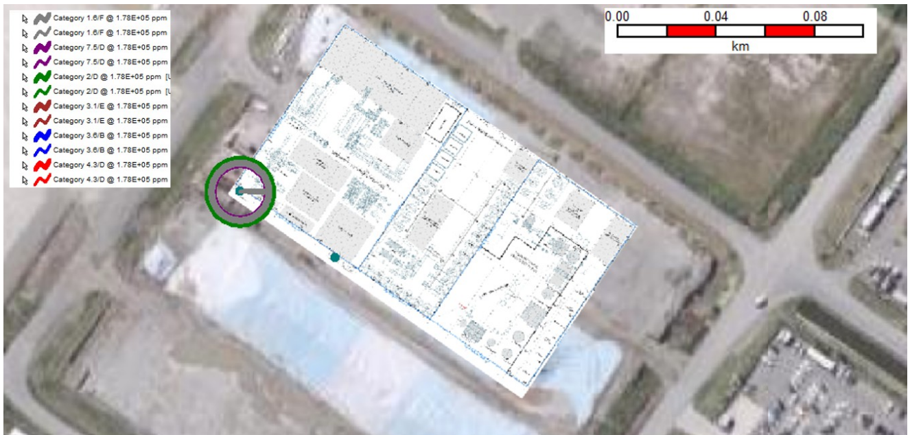
Figure 1: Oxygen Dispersion Contour to 35% Level for 25mm Hole Release
