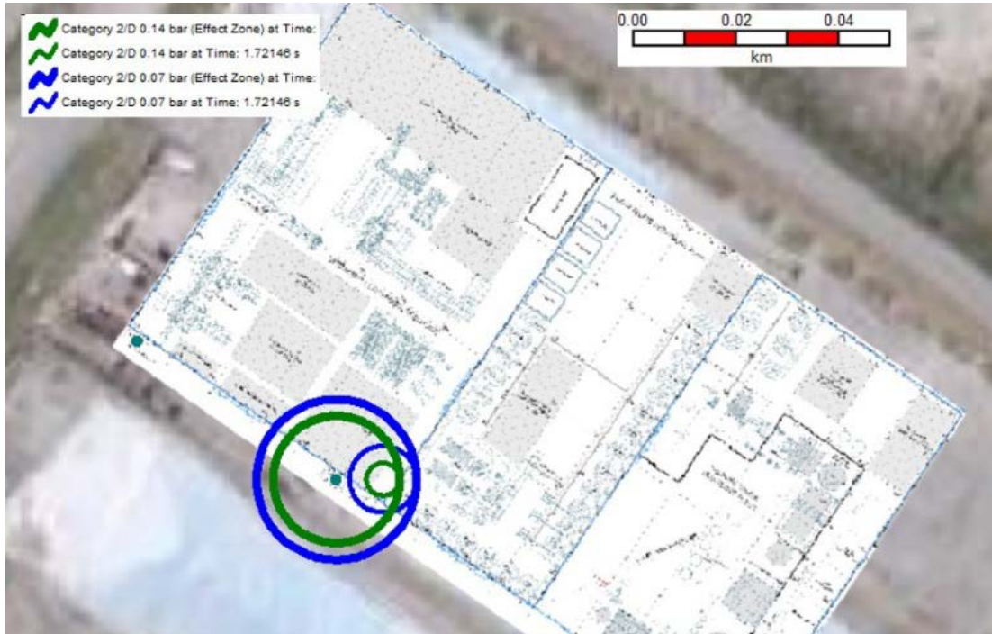
Figure 6: LPG 13mm release VCE Overpressure Contours
