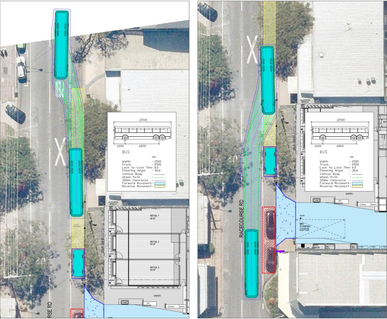
FIGURE 5.3 – SWEEP PATH OF BUS
