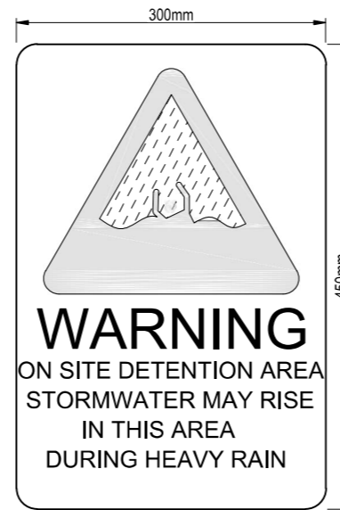
ON SITE STORMWATER DETENTION WARING SIGN
