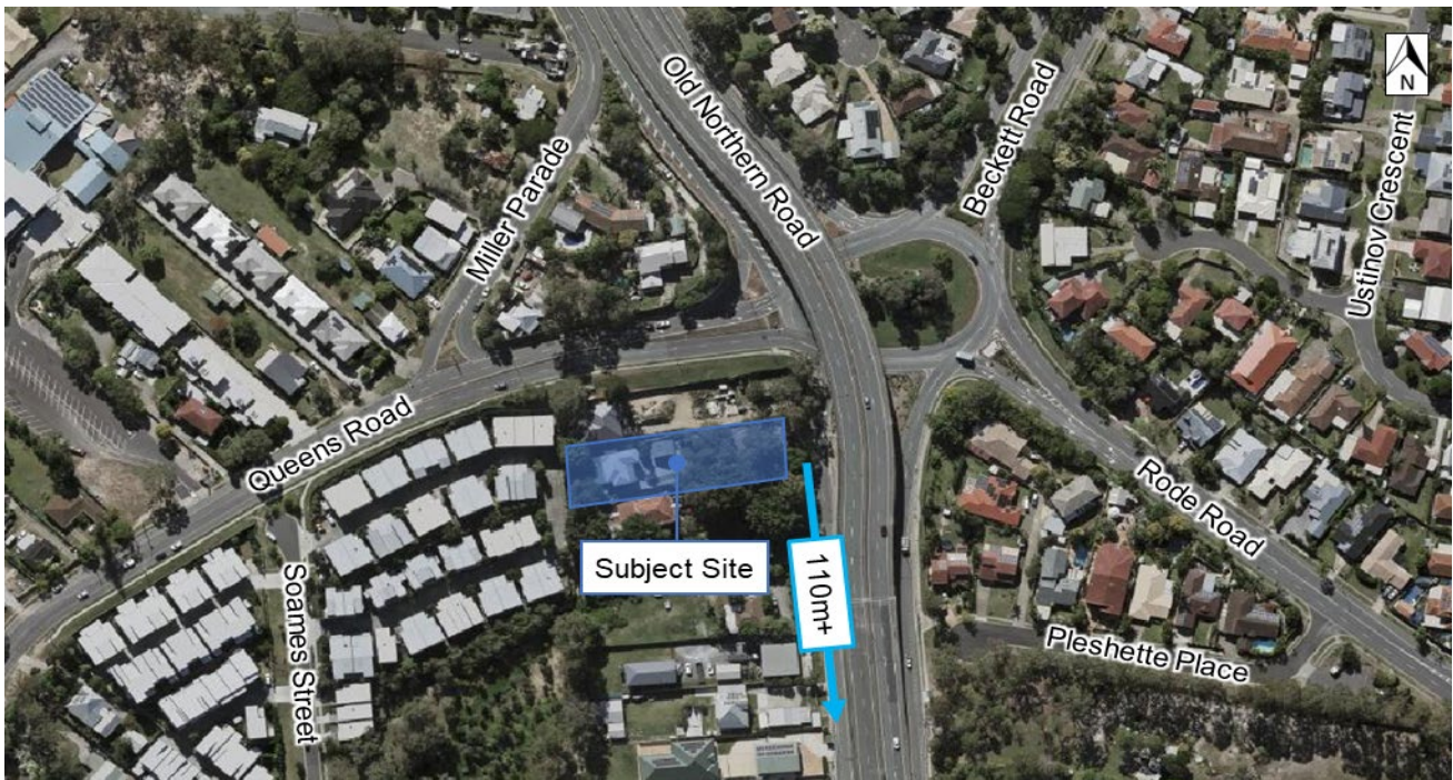
Figure 6.1: Available Sight Distance (Source: Queensland Globe)
