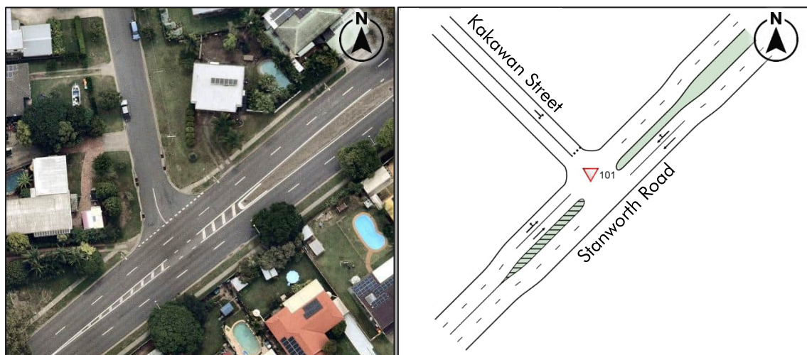
Figure 2.2: STANWORTH ROAD / KAKAWAN STREET INTERSECTION LAYOUT
