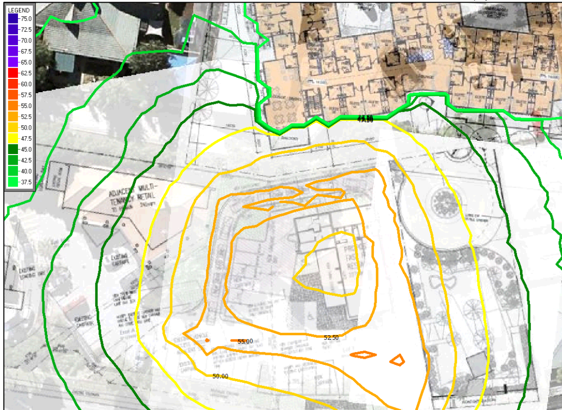
Plate B1: Noise contours at 8.1m (Level 3 height) – vehicle movements. Levels are in dB(A), L_{eq,adj,T}
