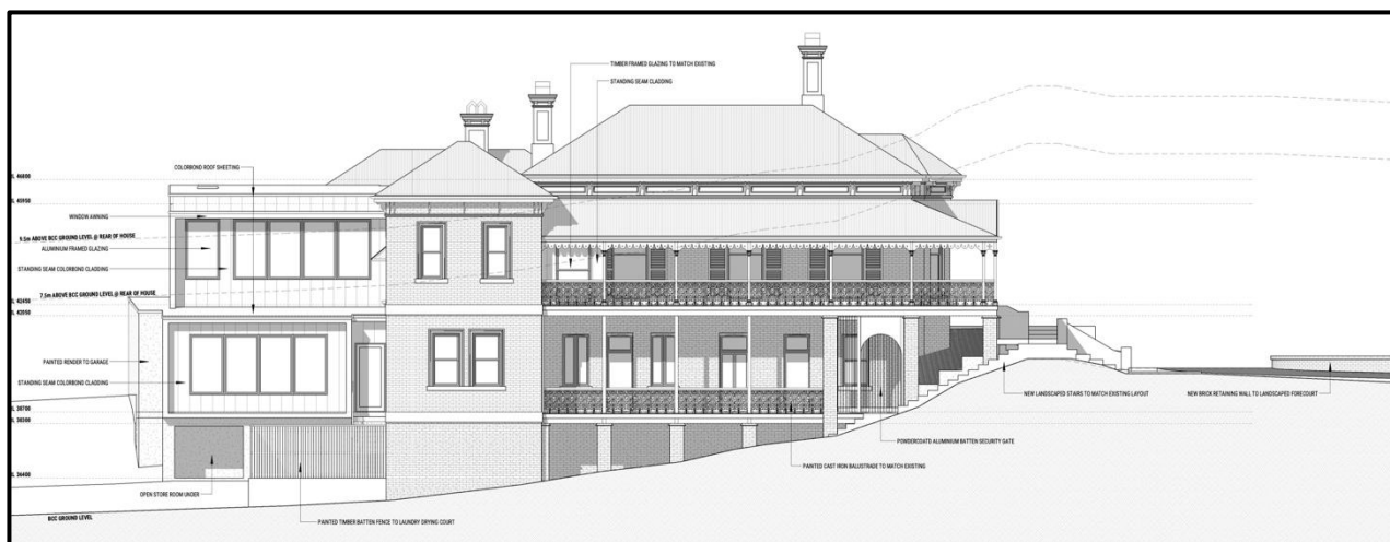
Demolition and proposed west elevation plan
