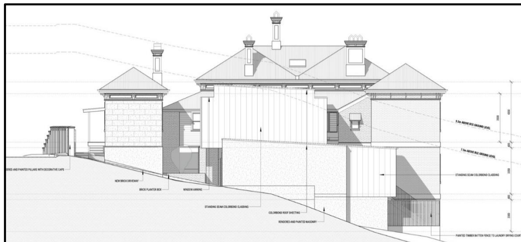
Demolition and proposed west elevation plan
