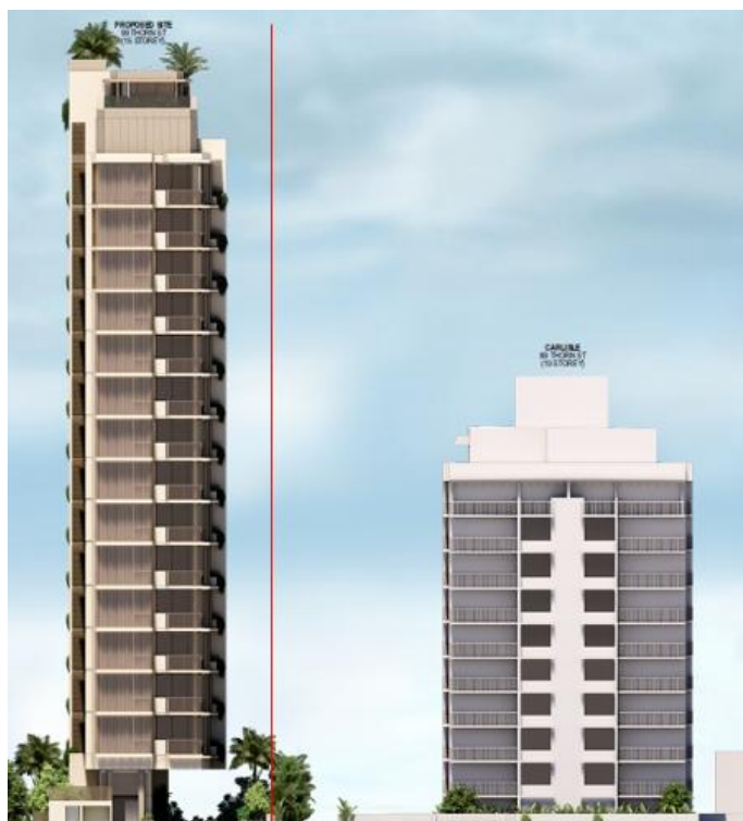
Figure 2 - Thorn Street Elevation demonstrating building setbacks.
