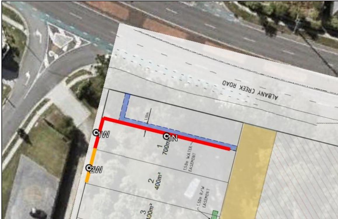
Plan B1: Showing the proposed location of the subdivision acoustic barriers on Lot 1, 2.
