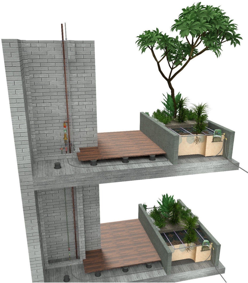
Figure 5 –Drip Irrigation - Multistorey Hydraulic Riser / Cupboard / Planter
