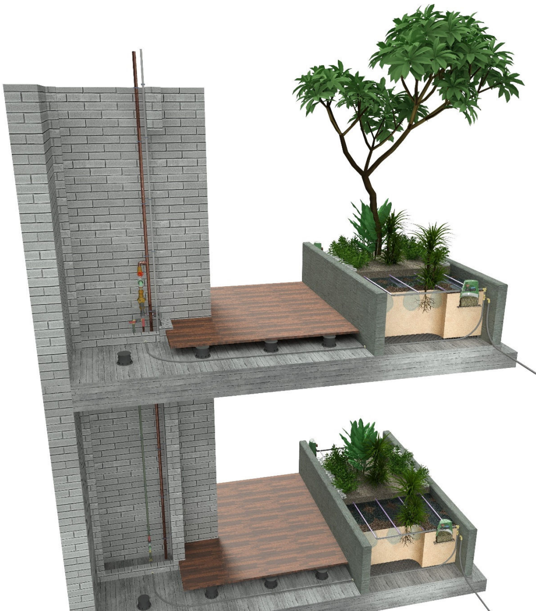
Figure 5 –Drip Irrigation - Multistorey Hydraulic Riser / Cupboard / Planter
