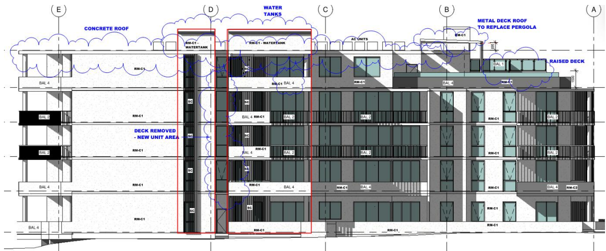
Figure 2: East elevation showing the continuation of projection elements up the building to the water tank level
