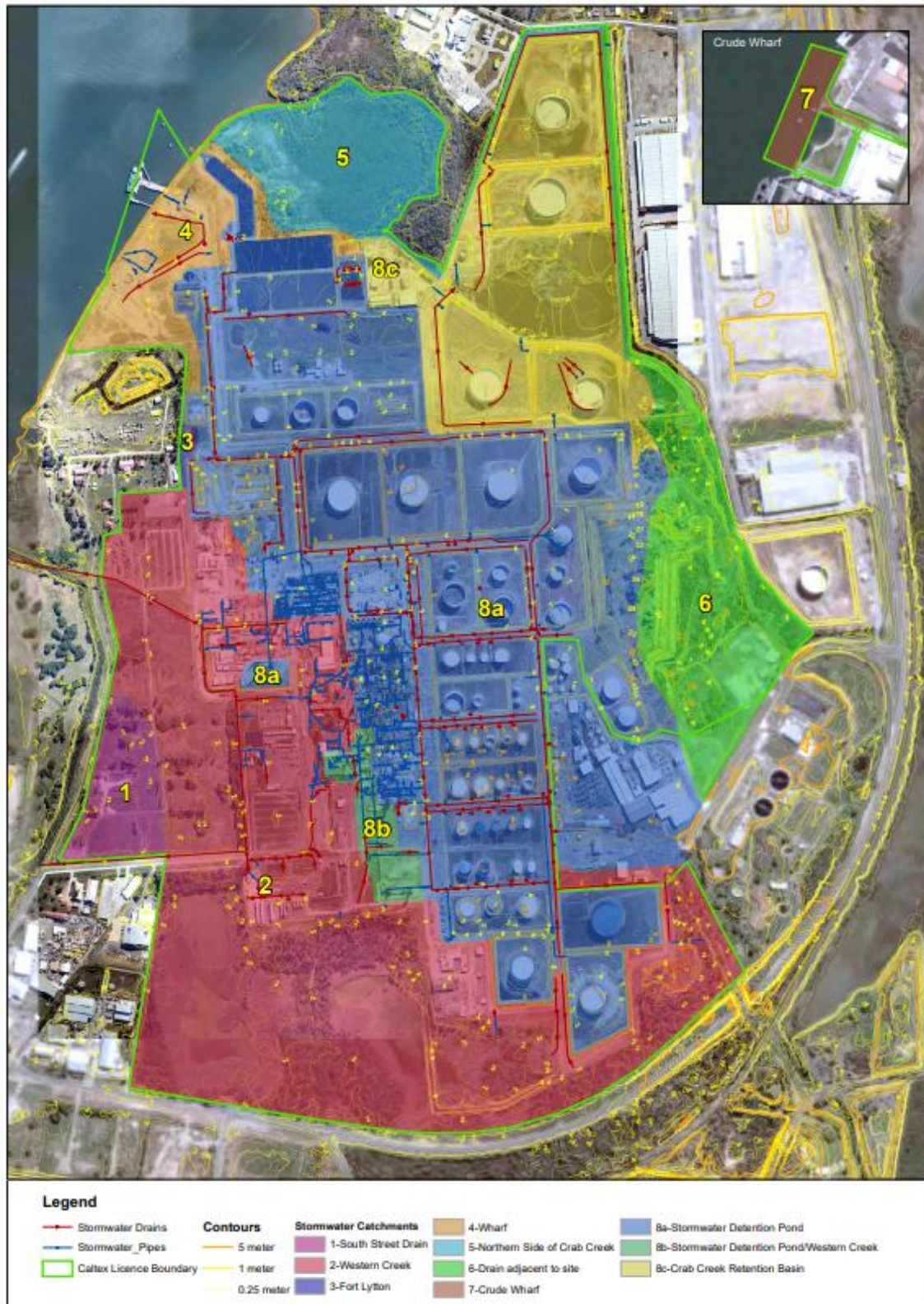
Figure 3-2 Existing Stormwater Catchments and Site Contours (Ampol, 2026)
