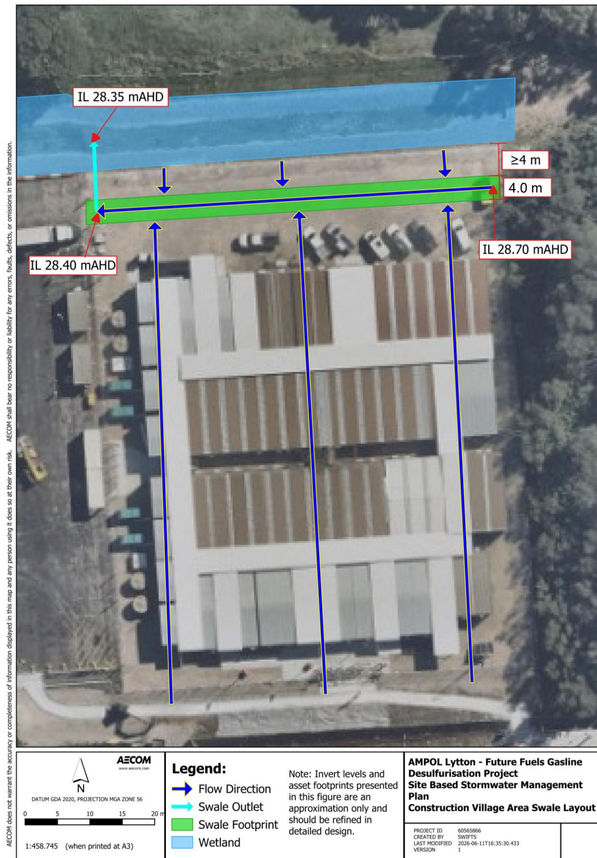
Figure 5-2: Construction Village area swale hypothetical arrangement
