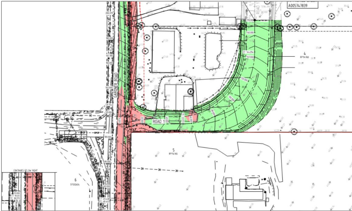
Figure 20: Modified intersection arrangement
