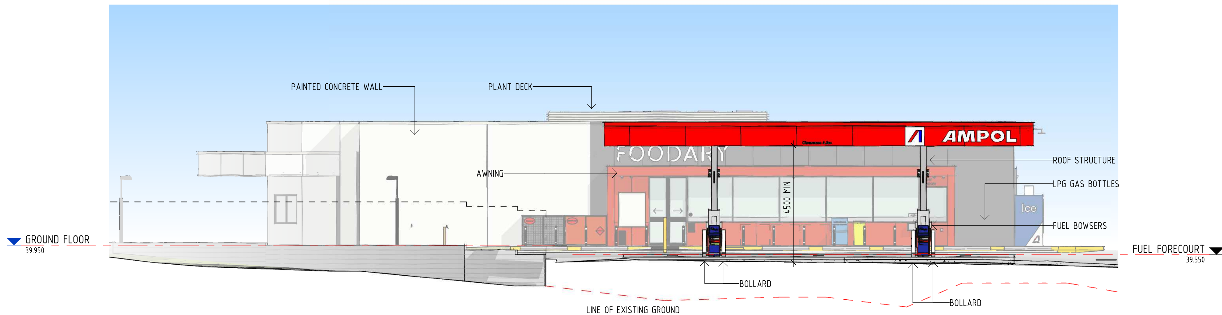
1 FUEL STATION NORTH ELEVATION 1 : 100
