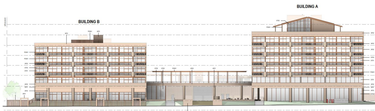
Figure 2. Northern elevation illustrating building height (Rothelowman)
