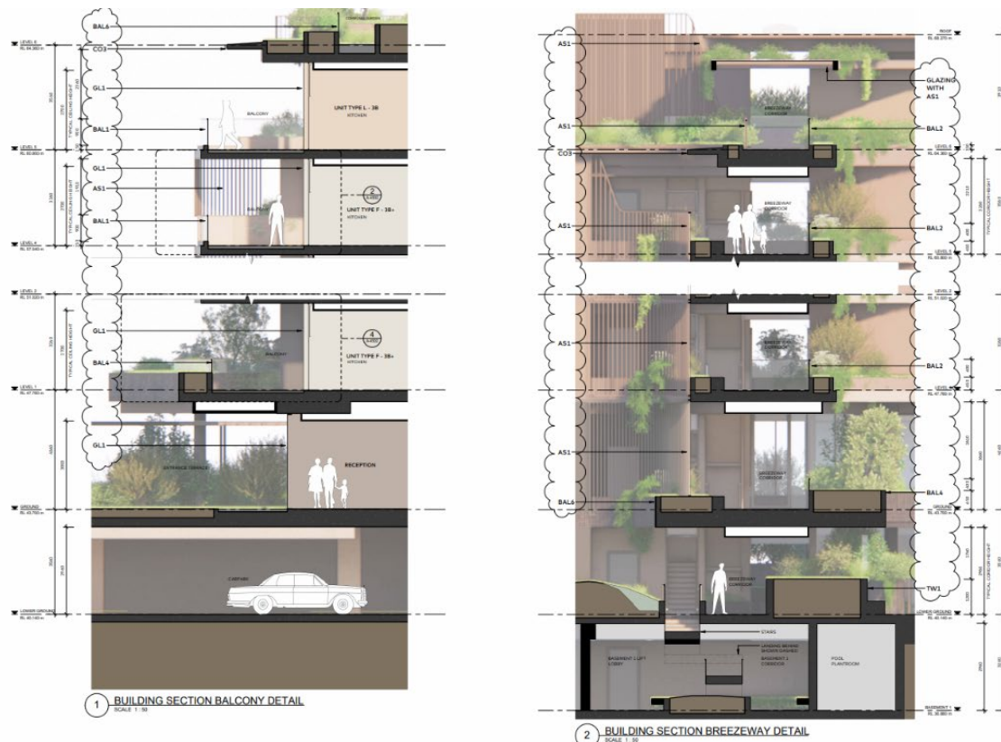
Figure 4 – Building Sections – Breezeway and Balconies
