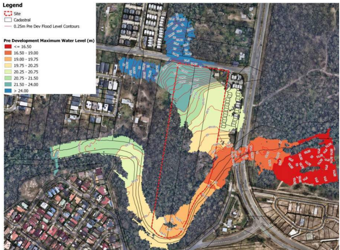
Figure 6: 2% AEP Pre Development Flood Levels
