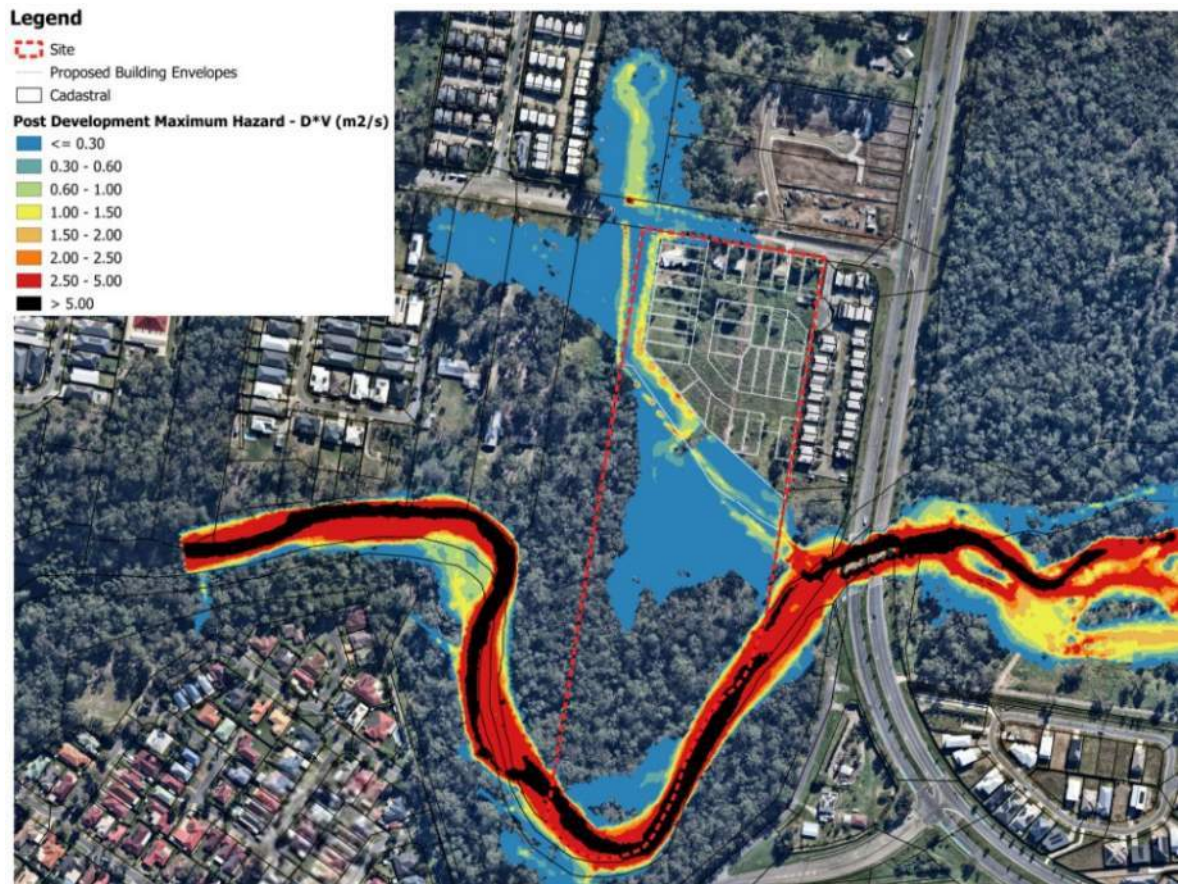
Figure 13: 2% AEP Post Development Hazard (D*V)
