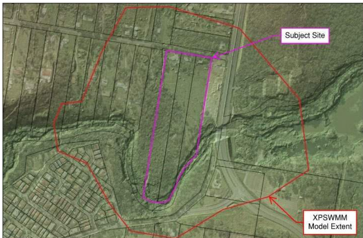
Figure 2: XP-SWMM Model Extent and DEM
