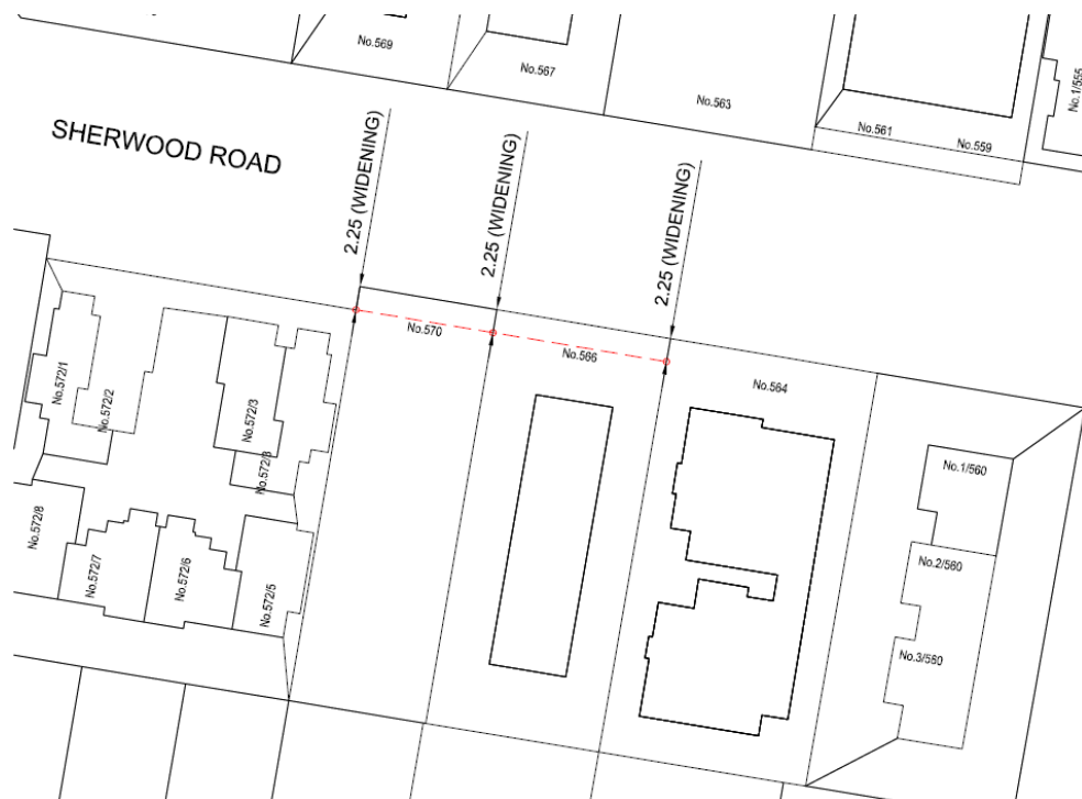
Figure 4: Sherwood Road - Road Widening
