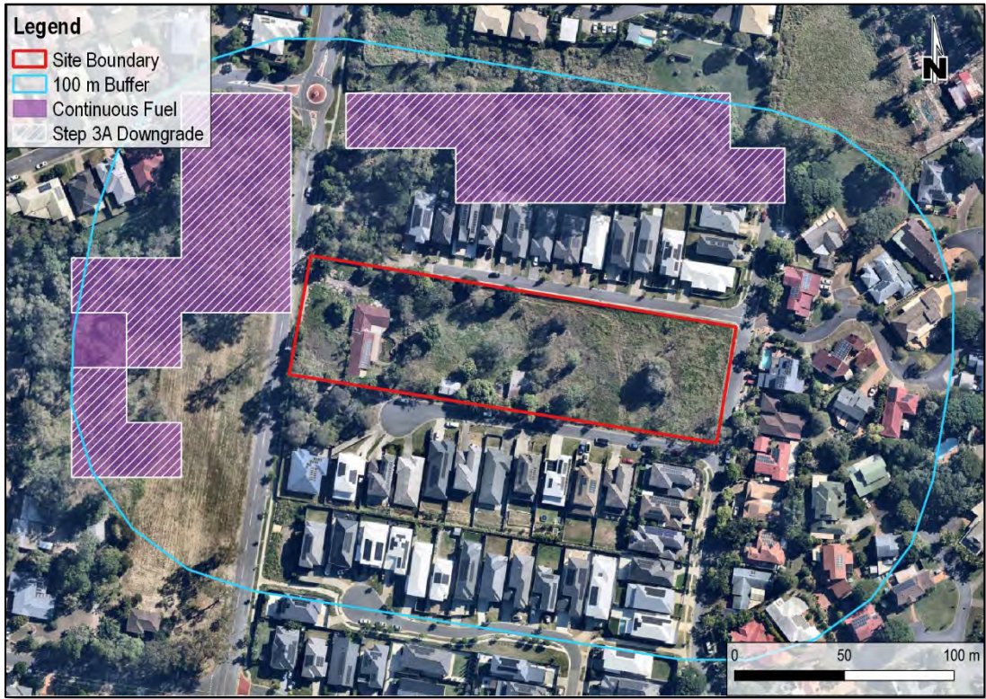
Figure 8. Shrinking of patches of continuous fuel at the interface with non-continuous fuel
