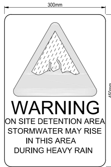
ON SITE STORMWATER DETENTION WARNING SIGN
