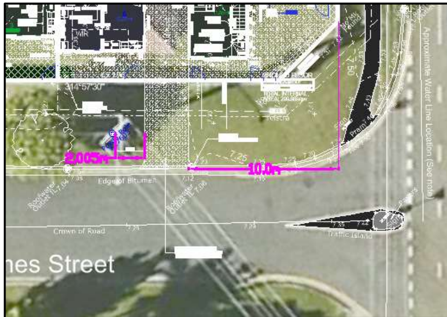
Figure 1: Location of driveway from intersection and power pole
