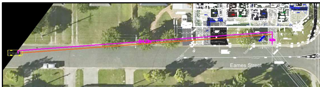
Figure 2: Sight distances to vehicles on Eames Road to the north
