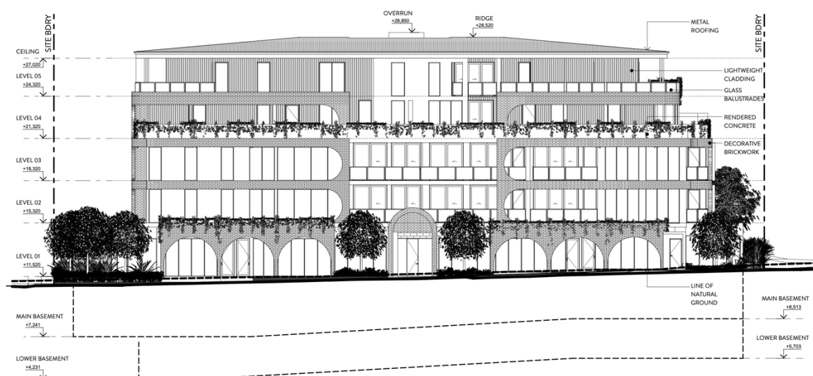
Figure 6: Extract of A006831135 Approved South Western Elevation
