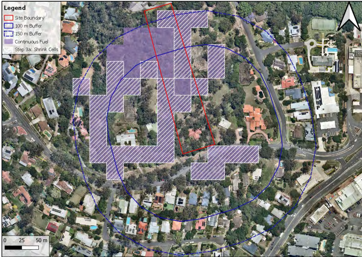
Figure 12. Shrinking of patches of continuous fuel at the interface with non-continuous fuel
