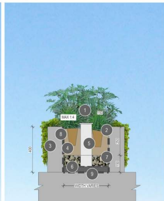
TYPICAL SHRUBS IN PODIUM DETAIL (MIN. 400mm DEEP) SCALE 1:10
