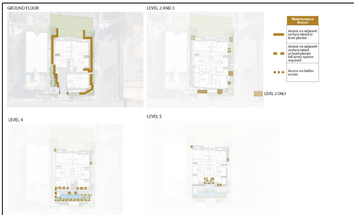
Figure 4: Maintenance Access Routes (Source: CUSP)
