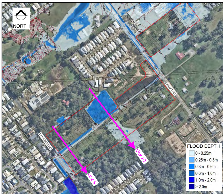
Figure 8 – Post-Development 2% AEP Overland Flow
