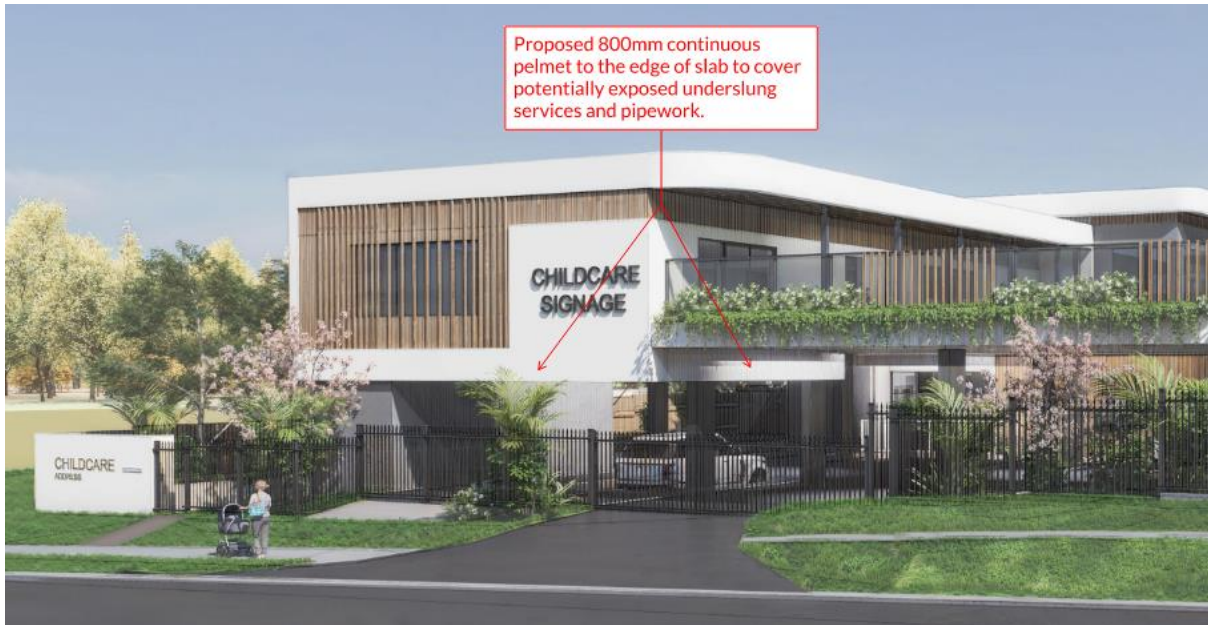
Figure 2: Artist's impressions of proposed revised continuous pelmet to cover potentially exposed underslung services and improve the perceived visual impact from Nottingham Road.
