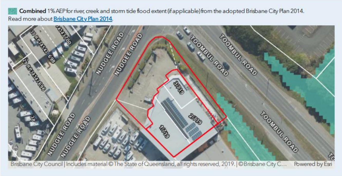
Above: Combined 1%AEP for river, creek and storm tide flood extent does not impact the existing building.
