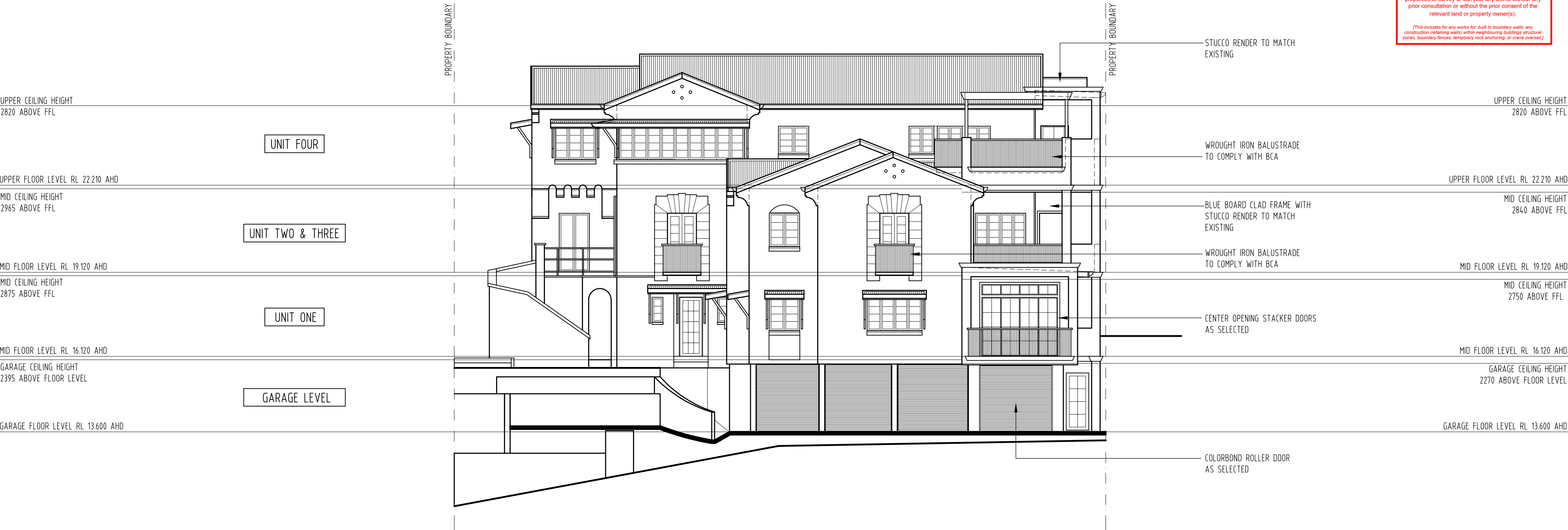
PROPOSED SOUTH ELEVATION
