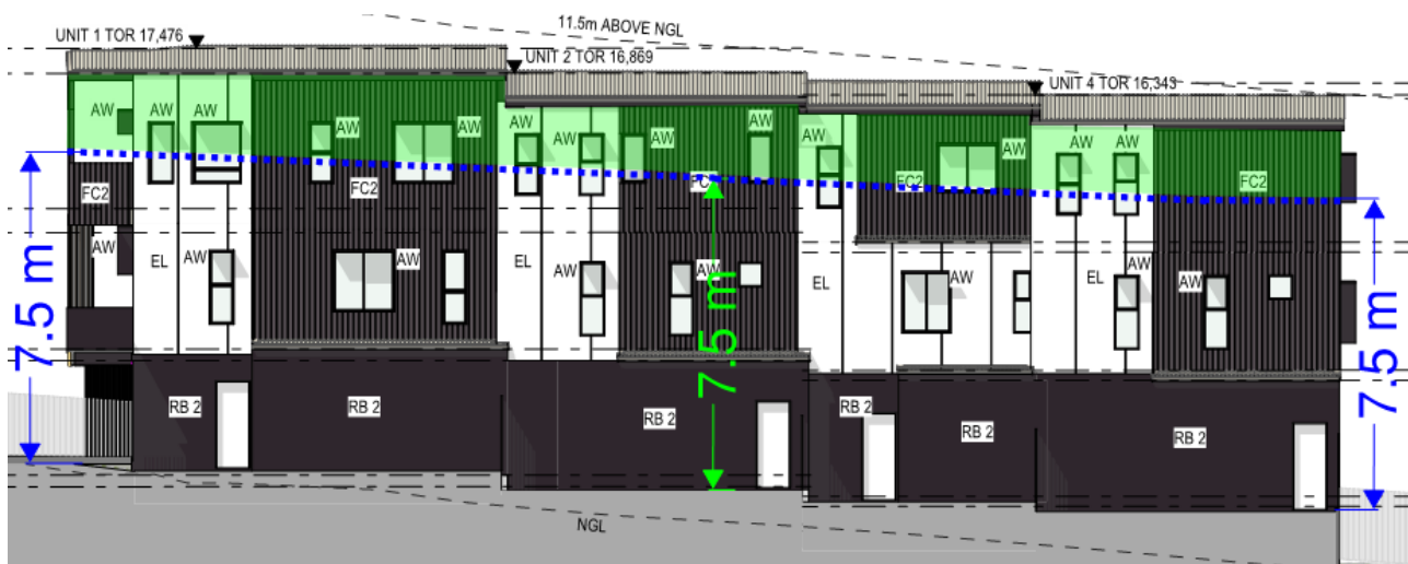
Figure 4: The non-compliance area shown in green.
