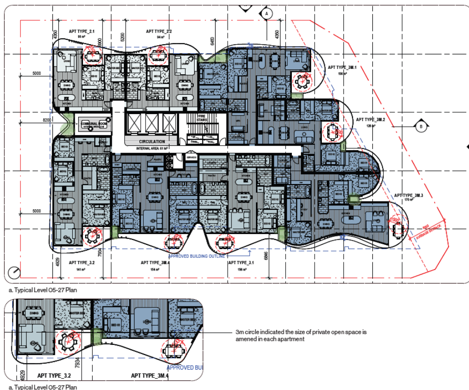
Figure 3: Plan Extract Showing Minimum 3m Dimension for all Private Open Space Areas – Plus Studio (March 2026)
