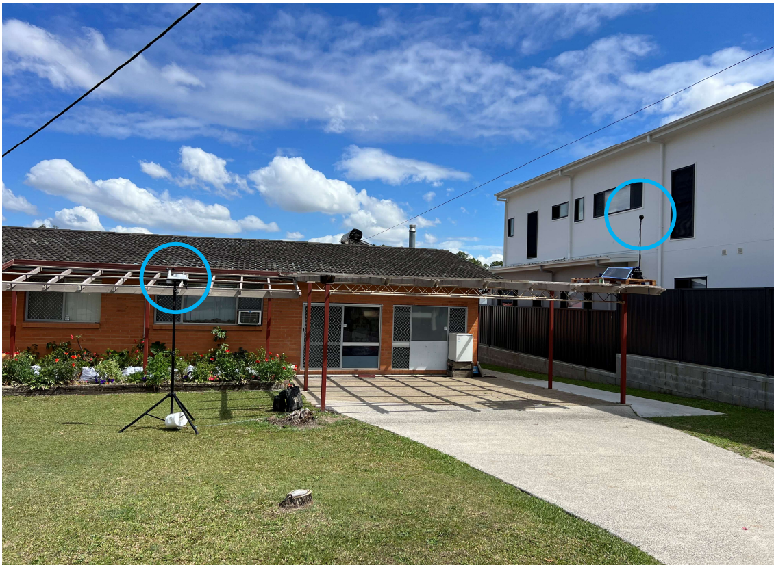
Image 5-1 Installed noise logger and weather station
