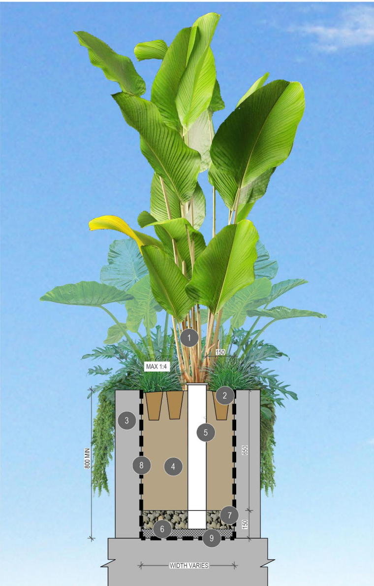
TYPICAL SHRUBS IN PODIUM DETAIL (MIN. 800mm DEEP) SCALE 1:10
