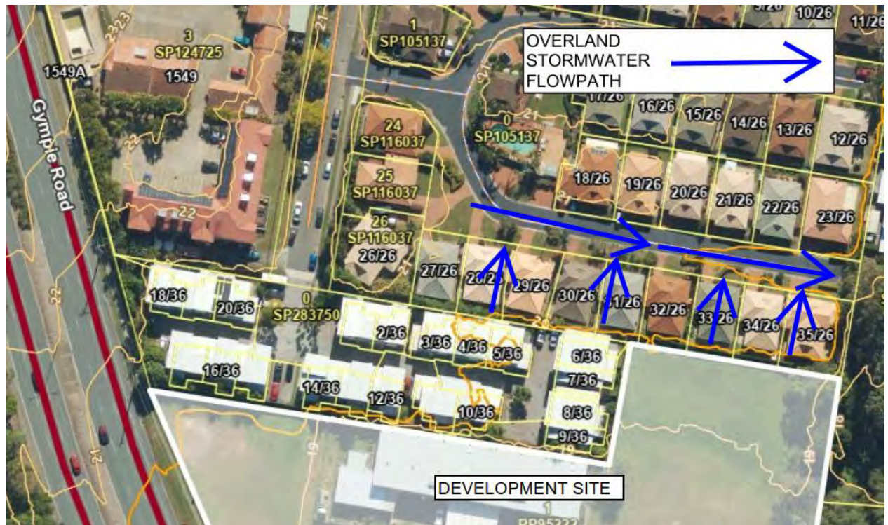
Figure 5: Existing Development Drainage Patterns (26 Stay Place)
