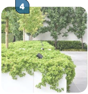
4 PODIUM PLANTERS Podium planters to develop green space away from 'natural ground'. Irrigation and drainage to all podium planter gardens to maximise plant growth
