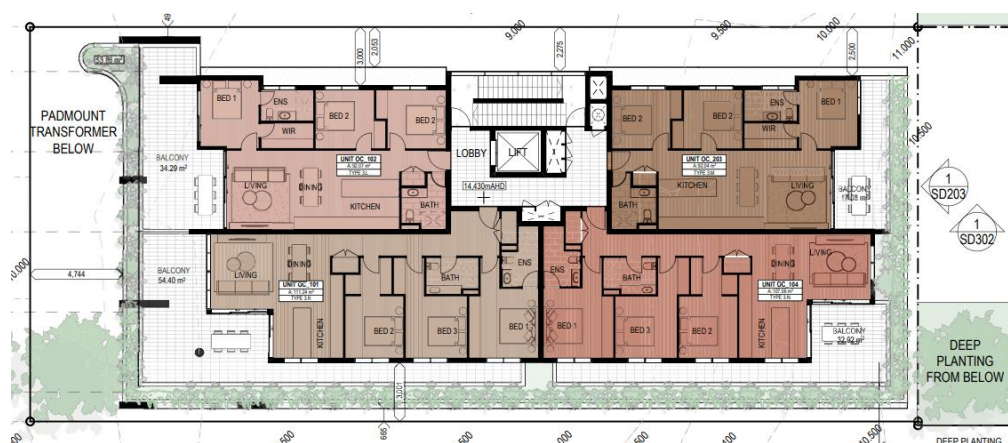
Figure 7: Proposed change to the Level 01 configuration (Source: DAH Architecture, 2026)
