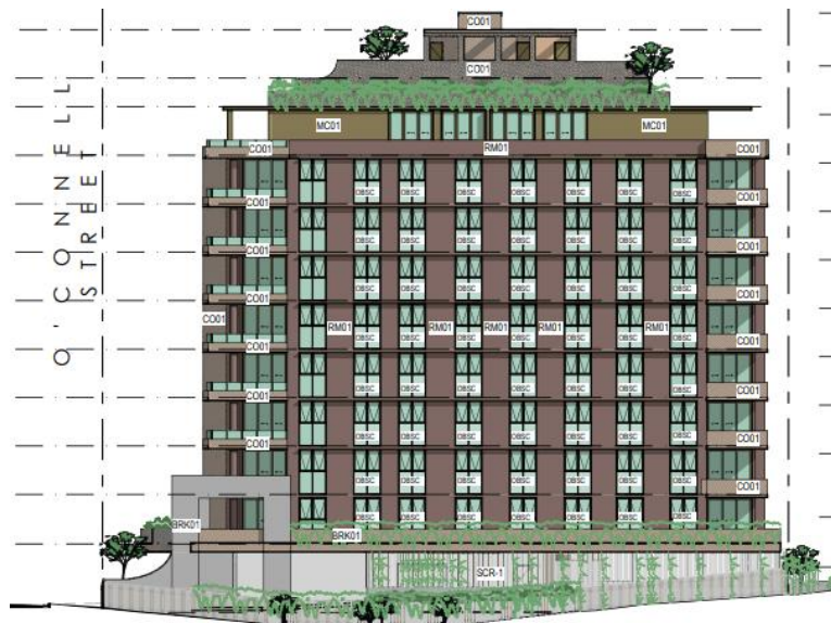
Figure 13: Proposed screening and landscaping outcome to car parking area - O'Connell St Tower (Source: DAH Architecture, 2026)
