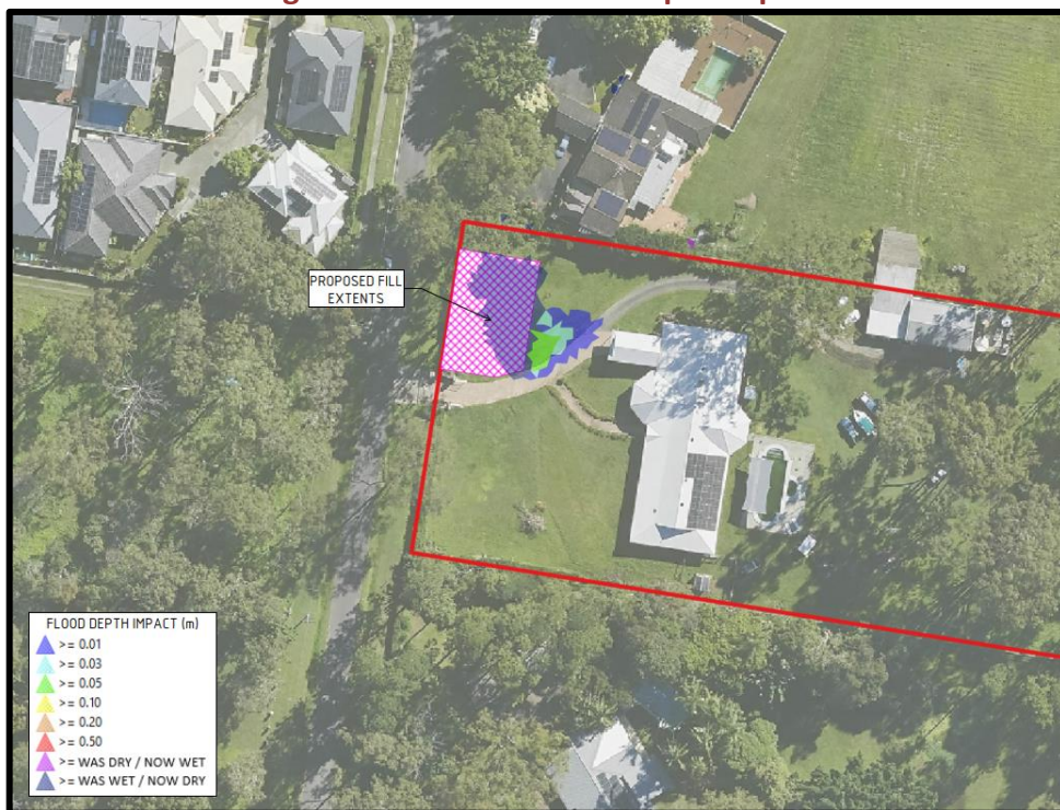
Figure 4.4: 1% AEP Flood Depth Impact
