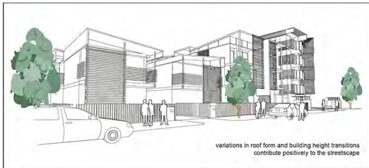
Figure m—Roof form
