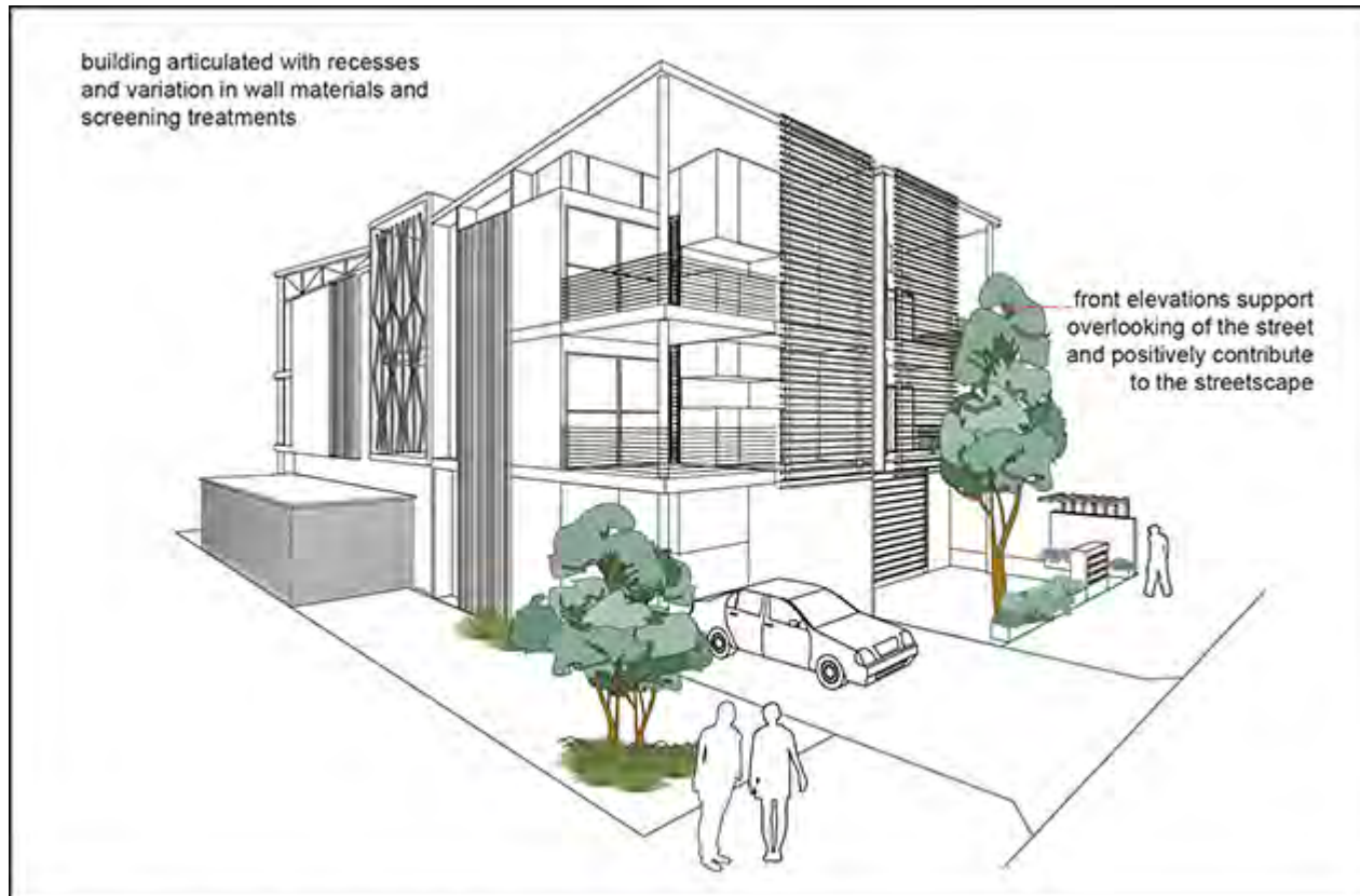
Figure i—Building length and depth articulation
