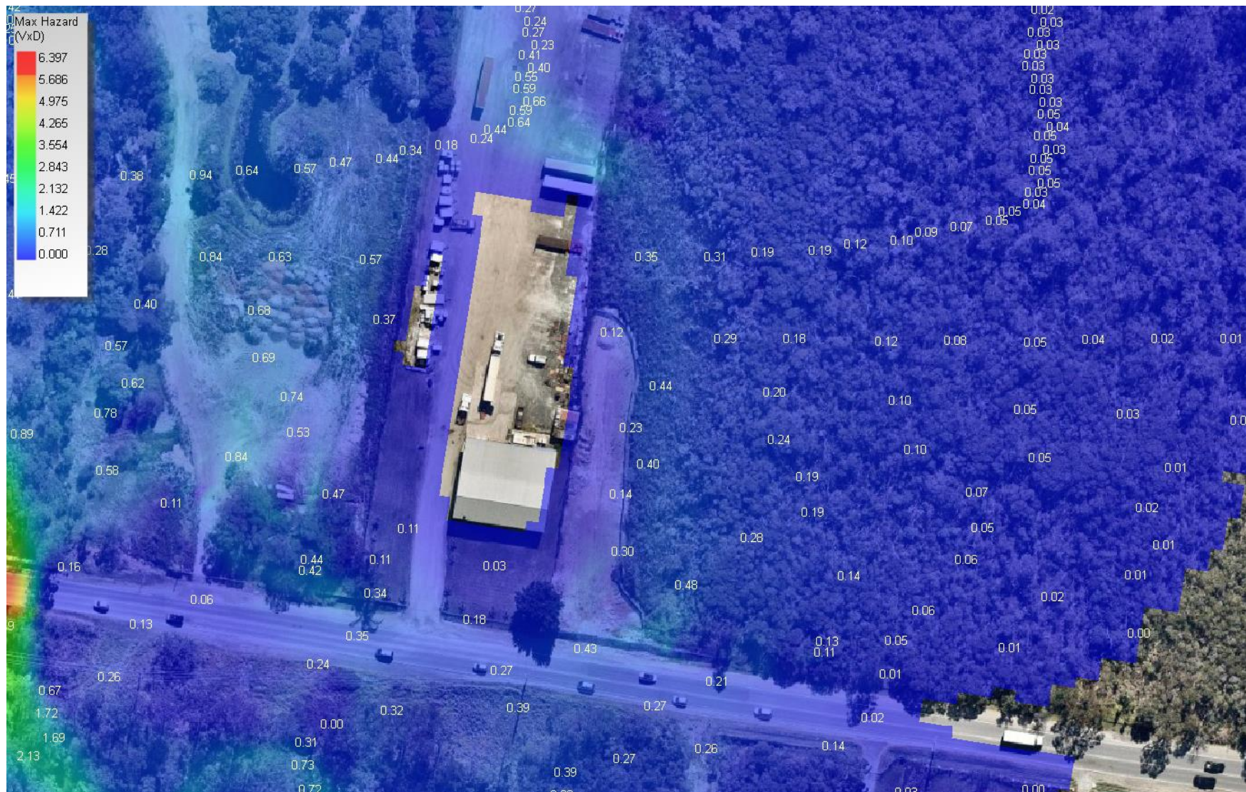
Figure E.3 – Flooding Hazards in a 1% AEP Event – Existing Condition
