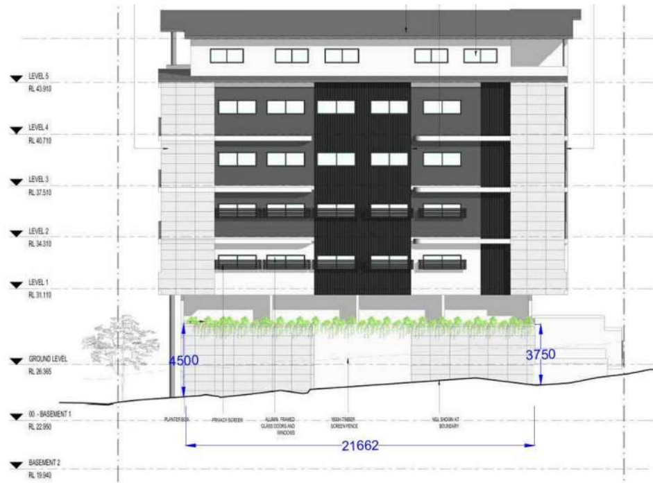
Figure 1 - Non-Compliant Built Boundary Wall (Western Elevation)
