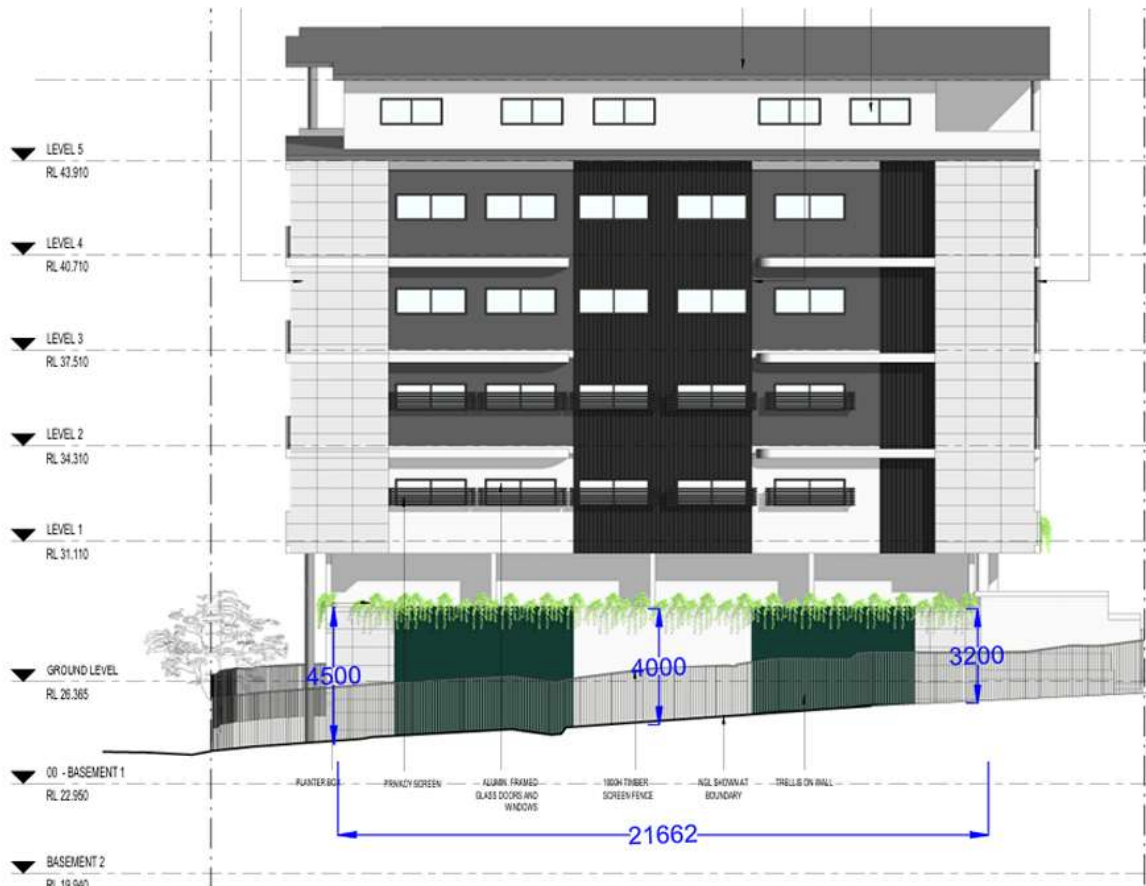
Figure 1 - Non-Compliant Built-to-Boundary Wall (Western Elevation – Amended Plans 1 May 2026)
