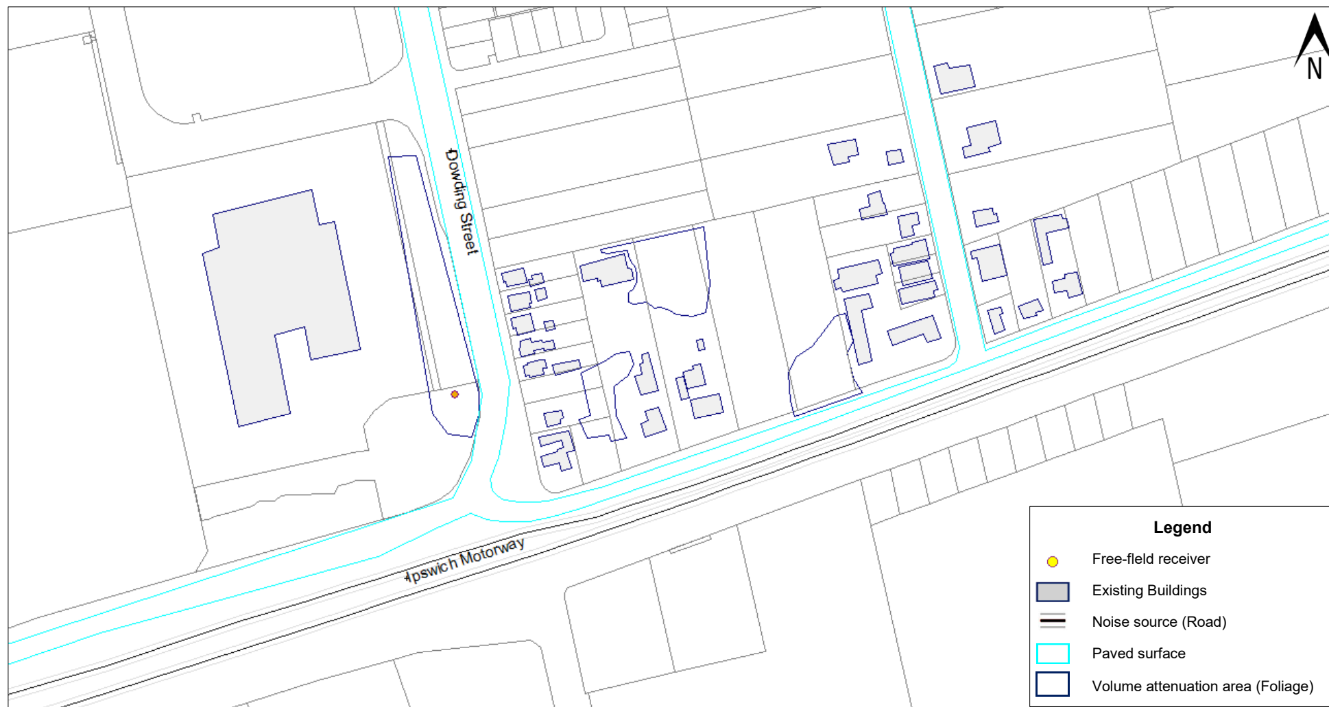
Figure 2.2 Excerpt from 3D SoundPLAN traffic noise validation model (year 2024)
