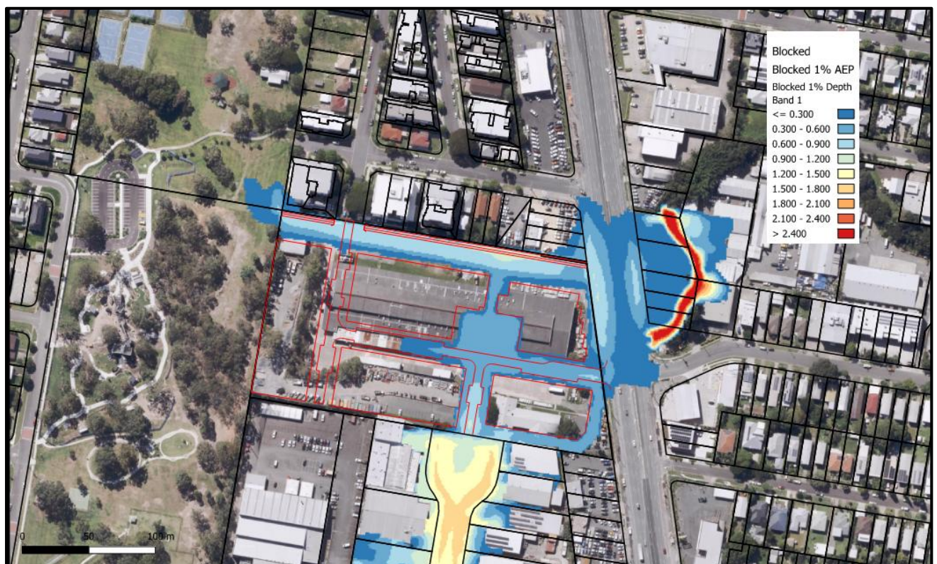
Figure 14: 100% Blocked 1% AEP Depth
