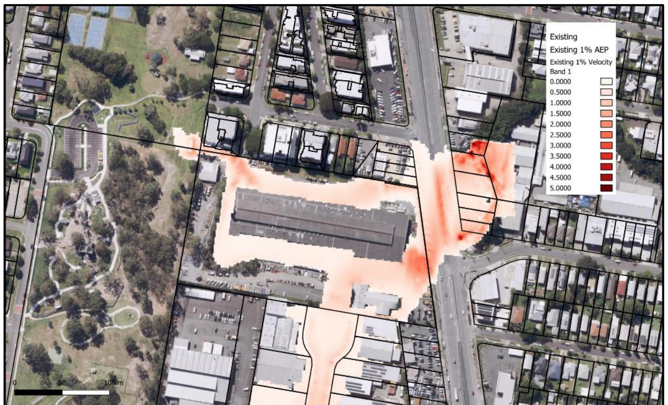
Figure 13: Existing 1% AEP Velocity
