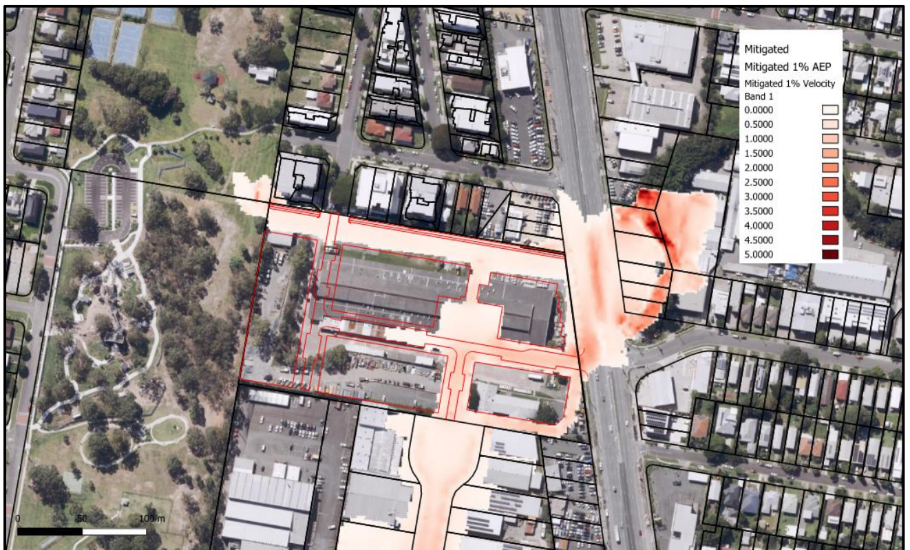
Figure 17: 50% Blocked Developed 1% Velocity
