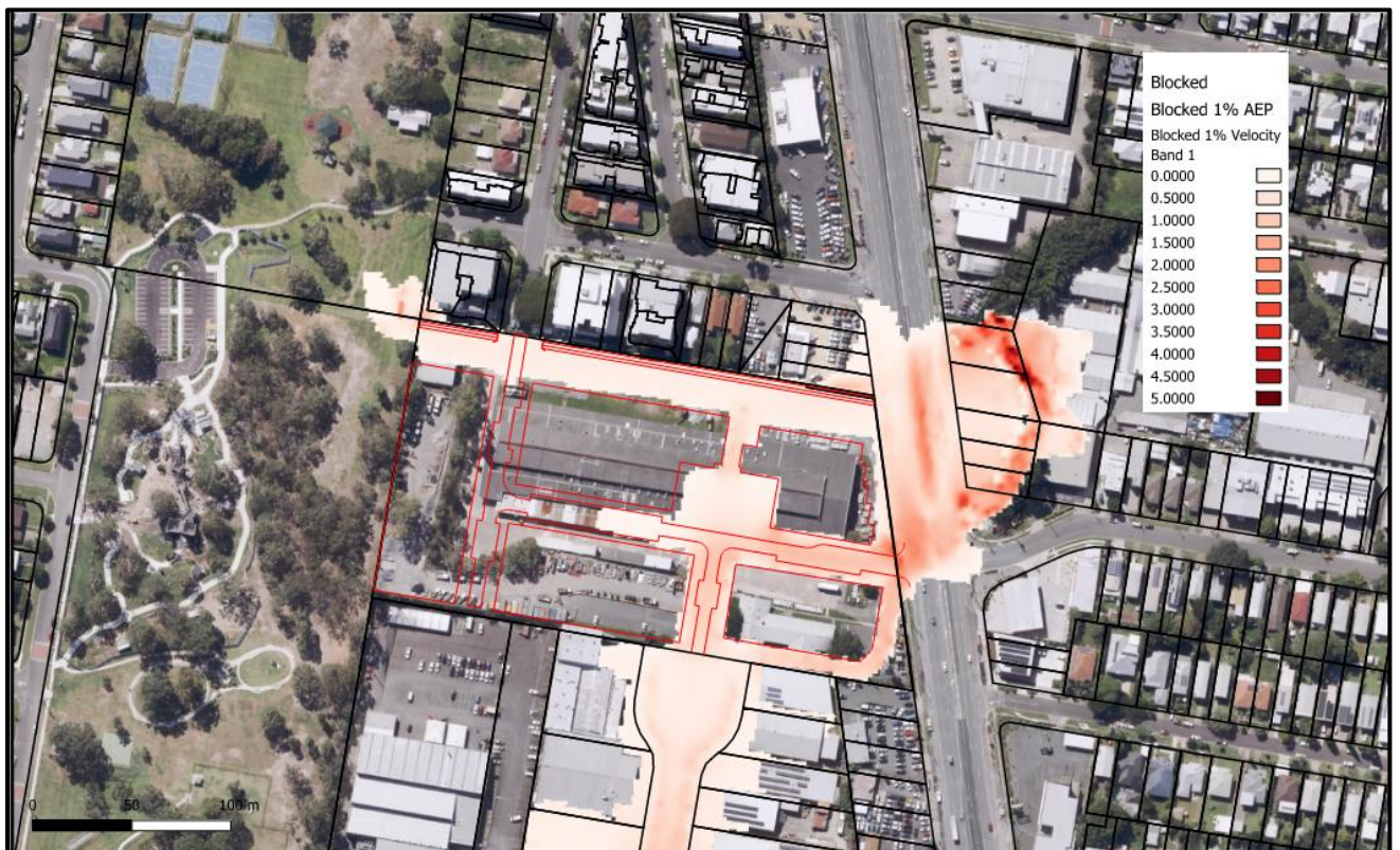
Figure 15: 100% Blocked Developed 1% AEP Velocity
