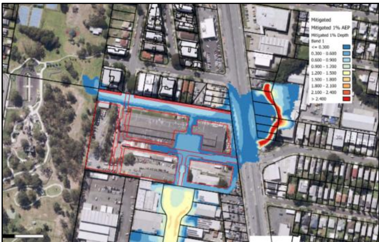
Figure 16: 50% Blocked Developed 1% AEP Depths
