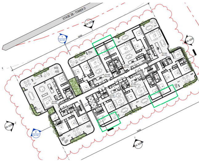
Picture 15 – Approved Level 11 Balcony Design (Emphasis in Green)
