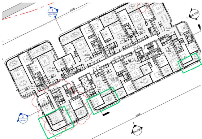
Picture 13 – Approved Levels 4-10 Balcony Design (Emphasis in Green)
