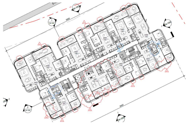
Picture 14 – Proposed Levels 4-10 Balcony Amendments (Clouded in Red)
