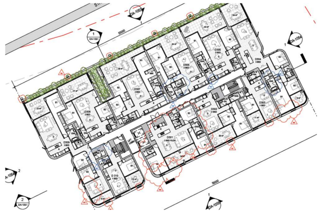
Picture 12 – Proposed Level 3 Balcony Amendments (Clouded in Red)
