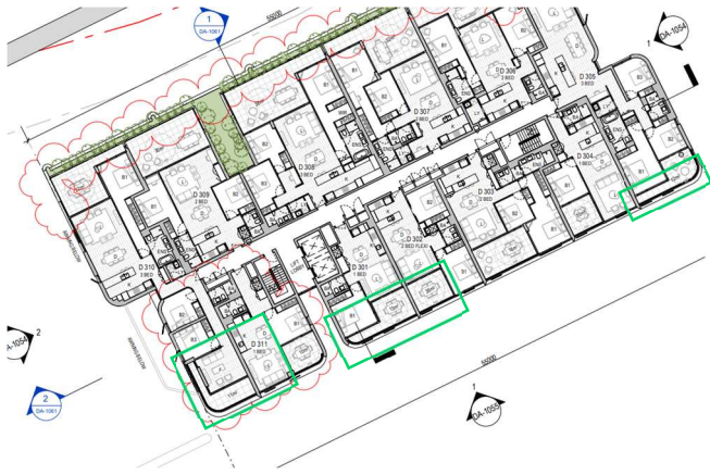
Picture 11 – Approved Level 3 Balcony Design (Emphasis in Green)
