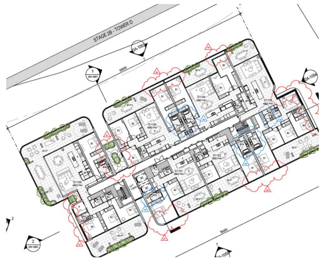
Picture 16 – Proposed Level 11 Balcony Amendments (Clouded in Red)
