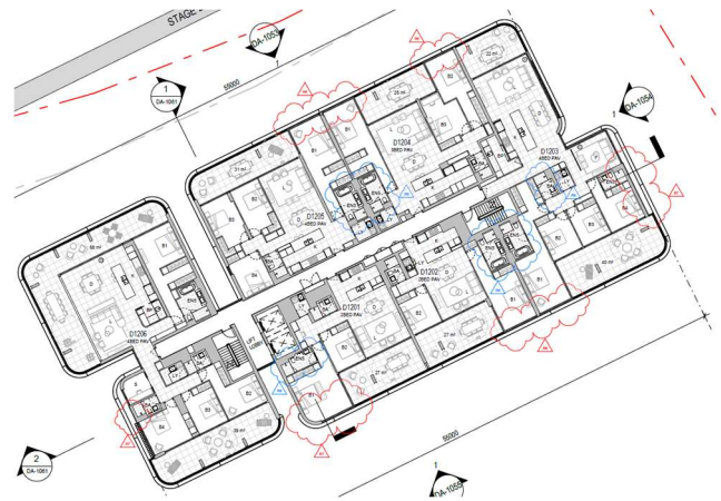
Picture 18 – Proposed Level 12-14 Balcony Amendments (Clouded in Red)
