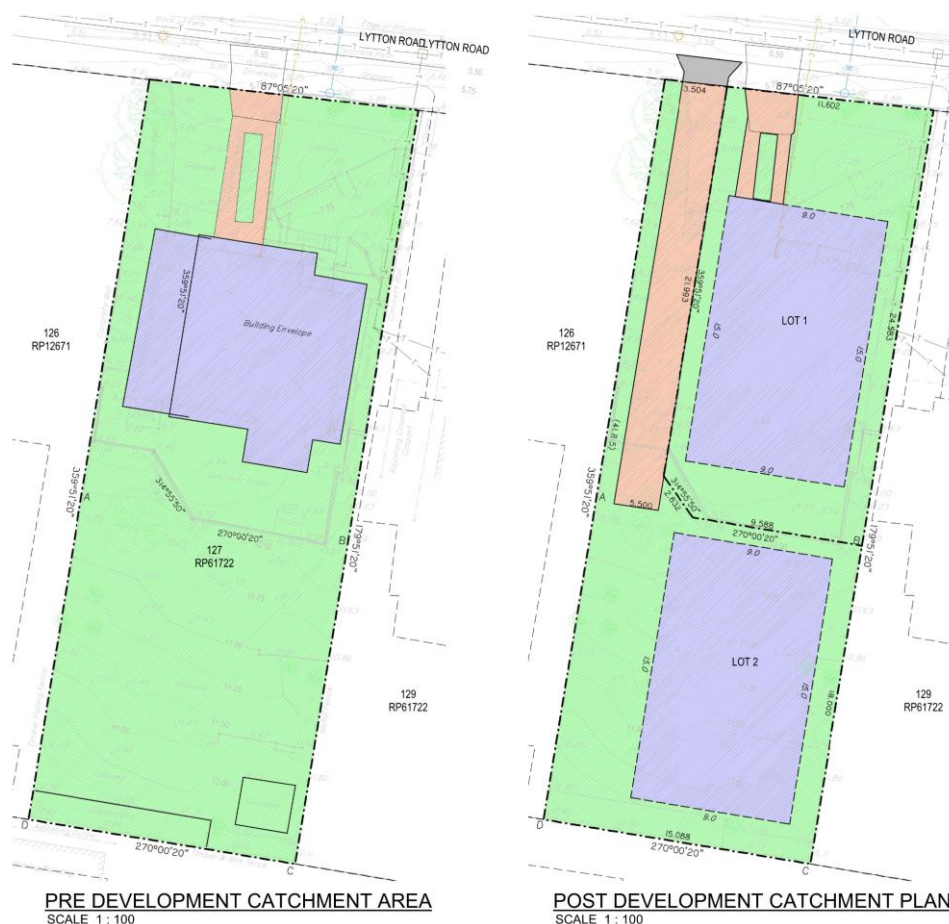
Figure 4: Pre-development and post-development stormwater catchment areas for the site at 107 Lytton Road, Bulimba, extracted from J.C. Engineers Civil Drawing D205_C_REV B_20260529.
