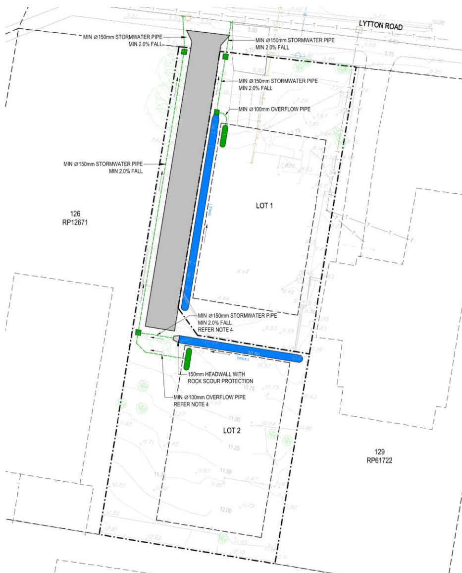
Figure 5: Stormwater Management Plan (Extracted from J.C.E. Civil Drawing D205_C_REV B_20260529, Sheet 7 of 7)
