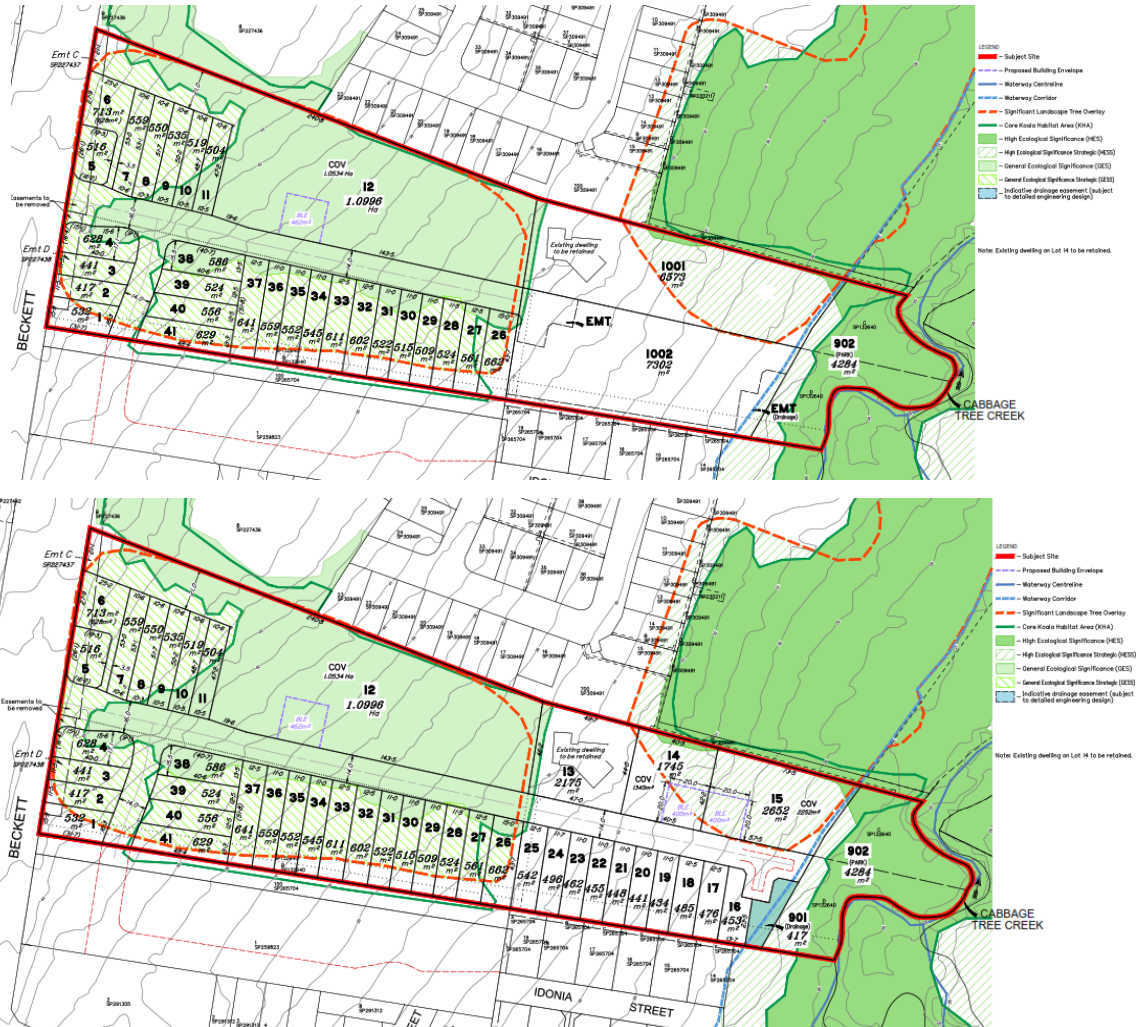
Figure 5 Proposed Subdivision Layout (Stage 1, Top and Stage 1 and 2, bottom) Source: DTS Group
