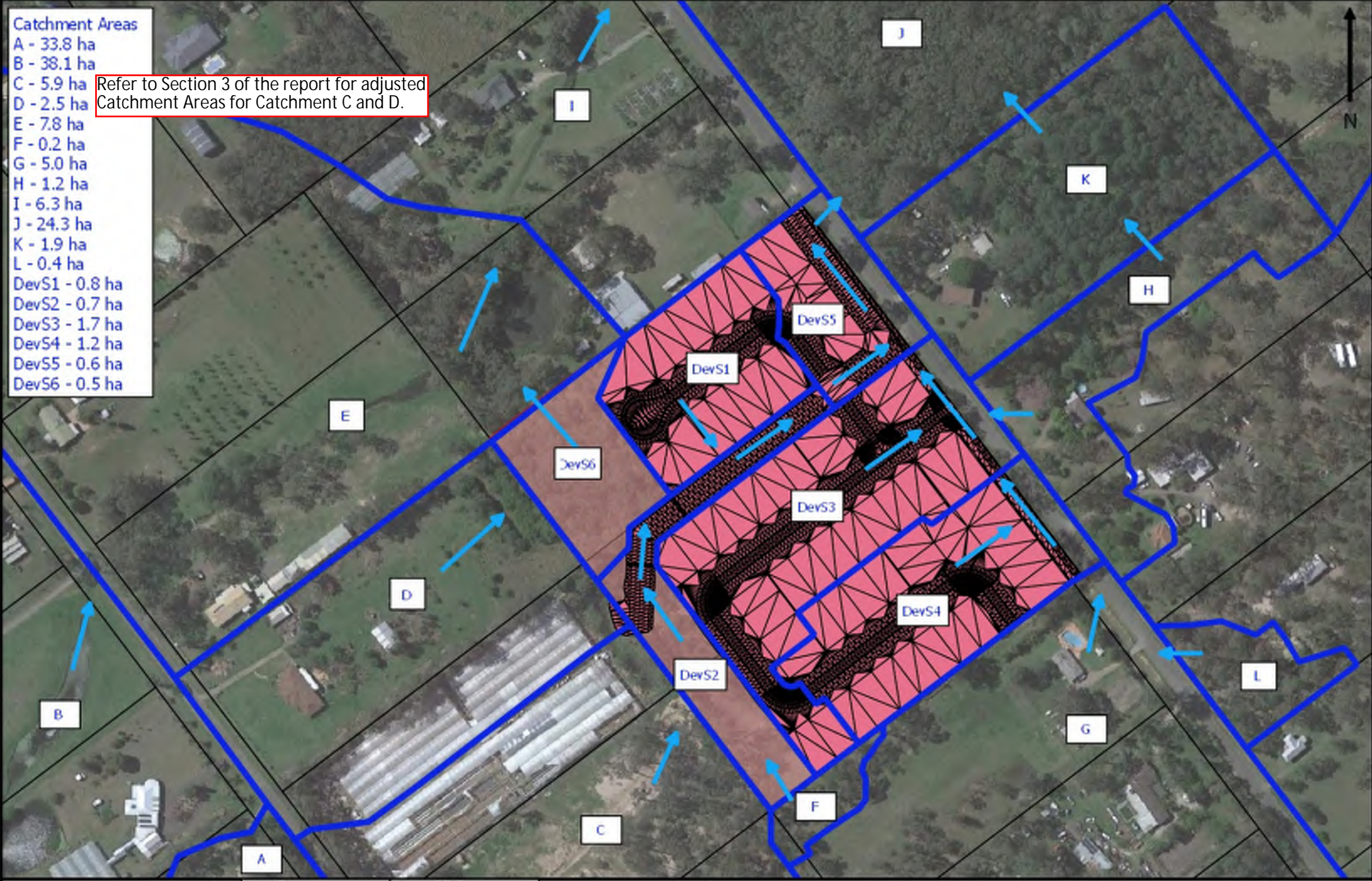
Figure 2B Developed Catchment Plan (Site close up)
