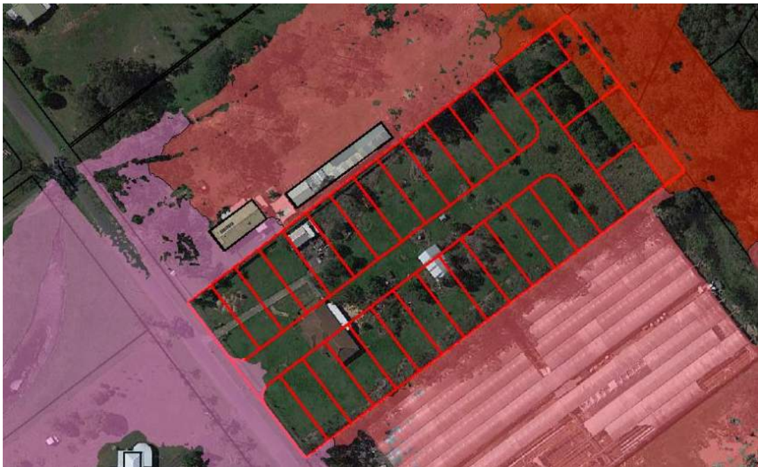
Figure 40 – Post-Development 2% AEP 60min water surface elevation in meters AHD (Site View)
