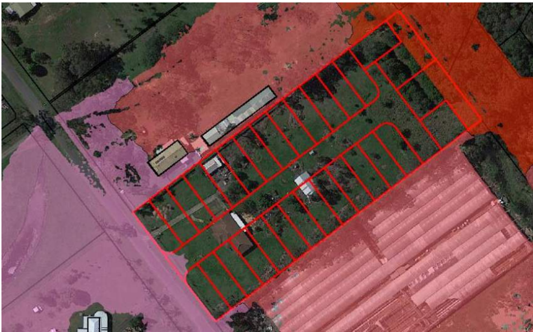
Figure 48 – Post-Development 2% AEP 90min water surface elevation in meters AHD (Site View)
