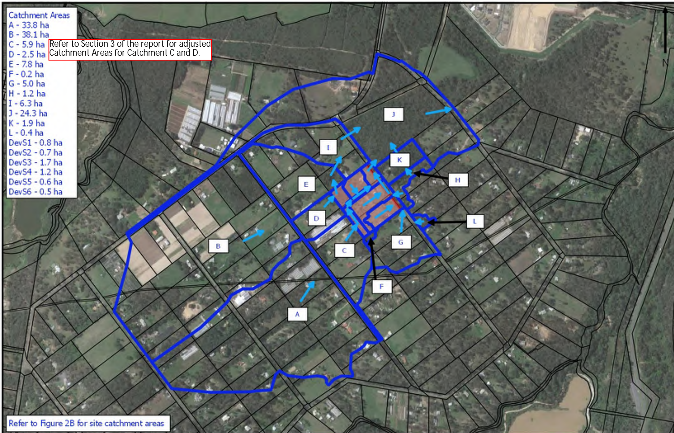
Figure 2A Developed Catchment Plan
