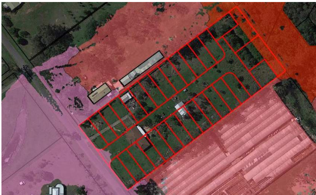
Figure 56 – Post-Development 2% AEP 120min water surface elevation in meters AHD (Site View)
