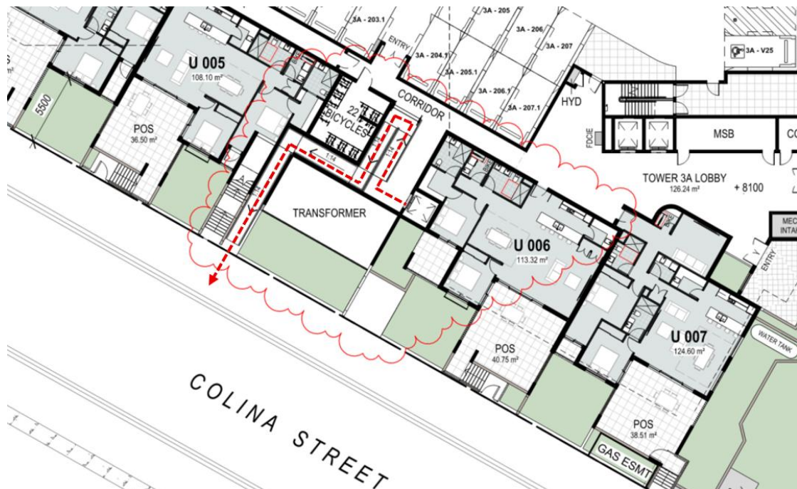
Figure 1: Ramped Pathway to lift access to Podium level
