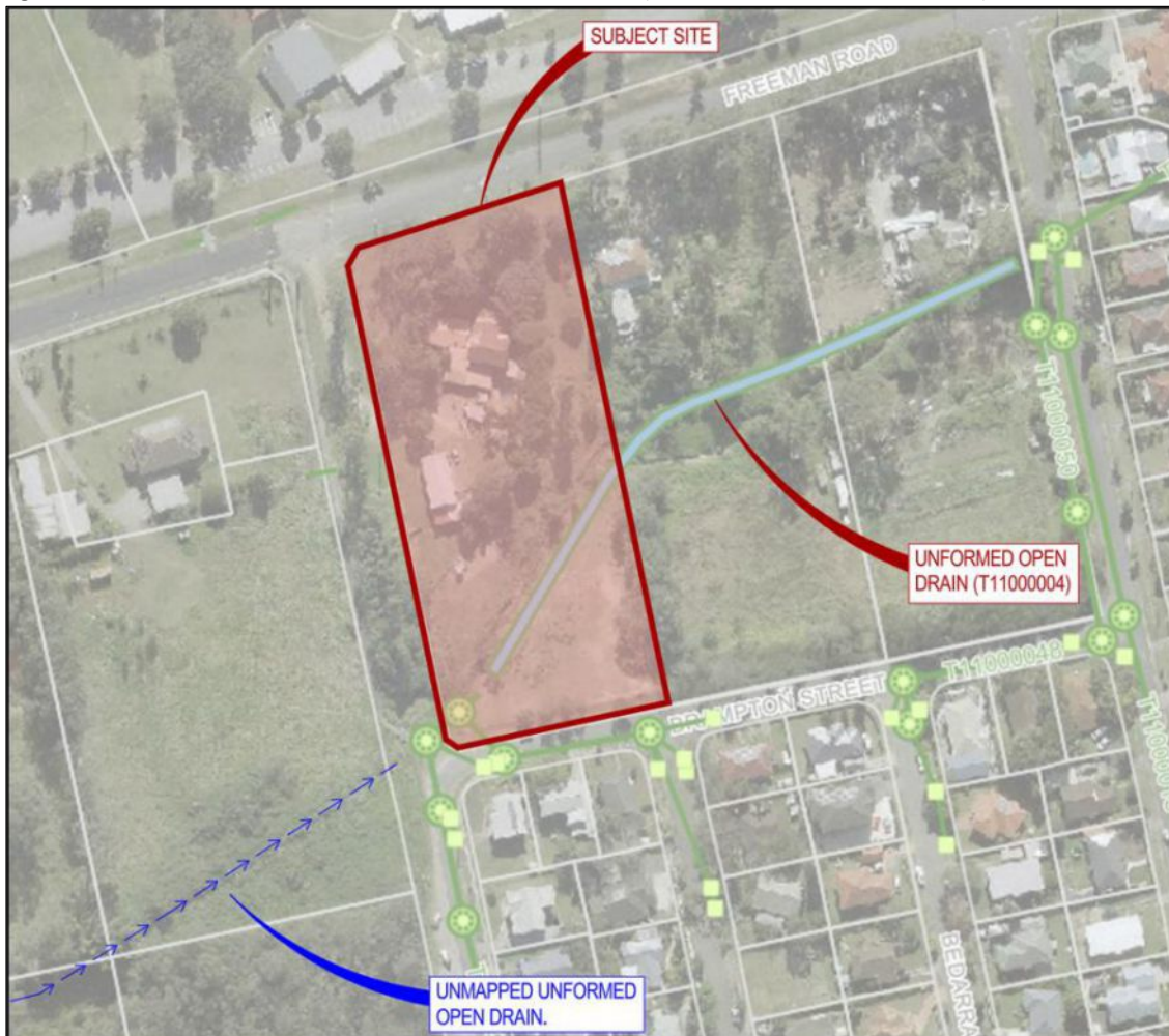
Figure 3-3 EXISTING STORMWATER INFRASTRUCTURE (BCC INFRASTRUCTURE MAPPING)
