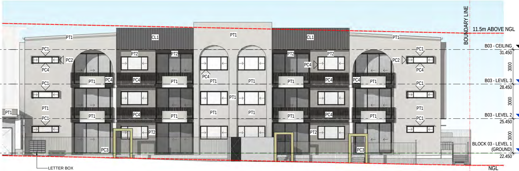
③ BLOCK 03 ELEVATION - EAST (WEBSTER RD) SCALE: 1 : 100 (@ A1)
