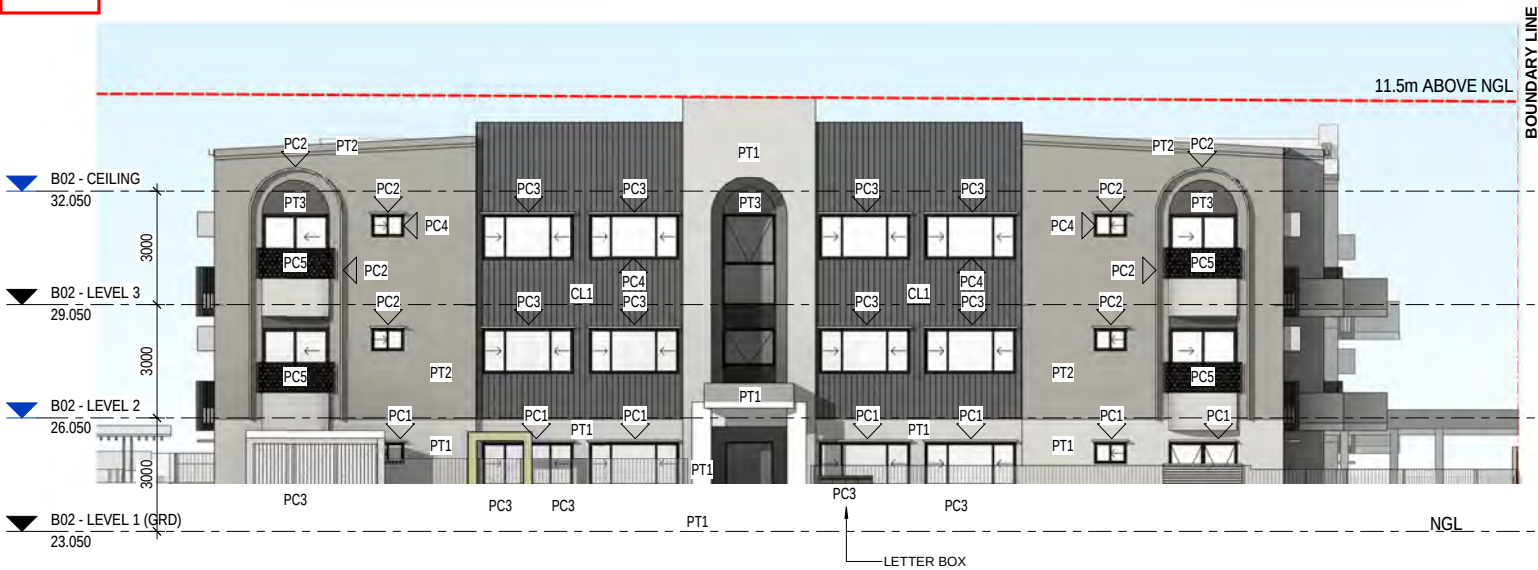
① BLOCK 02 ELEVATION - SOUTH (LINLEY ST.) SCALE: 1 : 100 (@ A1)
