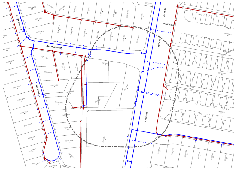
Figure 7 - Water Main (Blue) and Sewer Main (Red)
