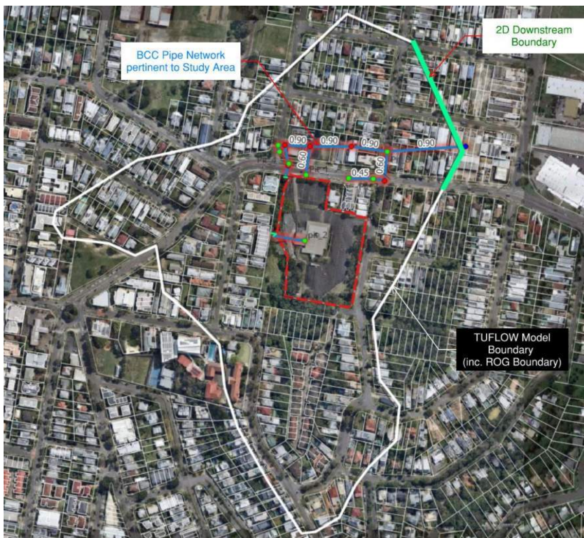
Figure 8 – TUFLOW model Setup – MPN Pre-development scenario
