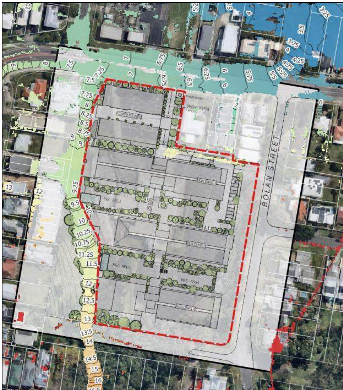
Figure 12 – 2% AEP Flood Levels – Post-Development Case w/ Proposed Concept Plan
