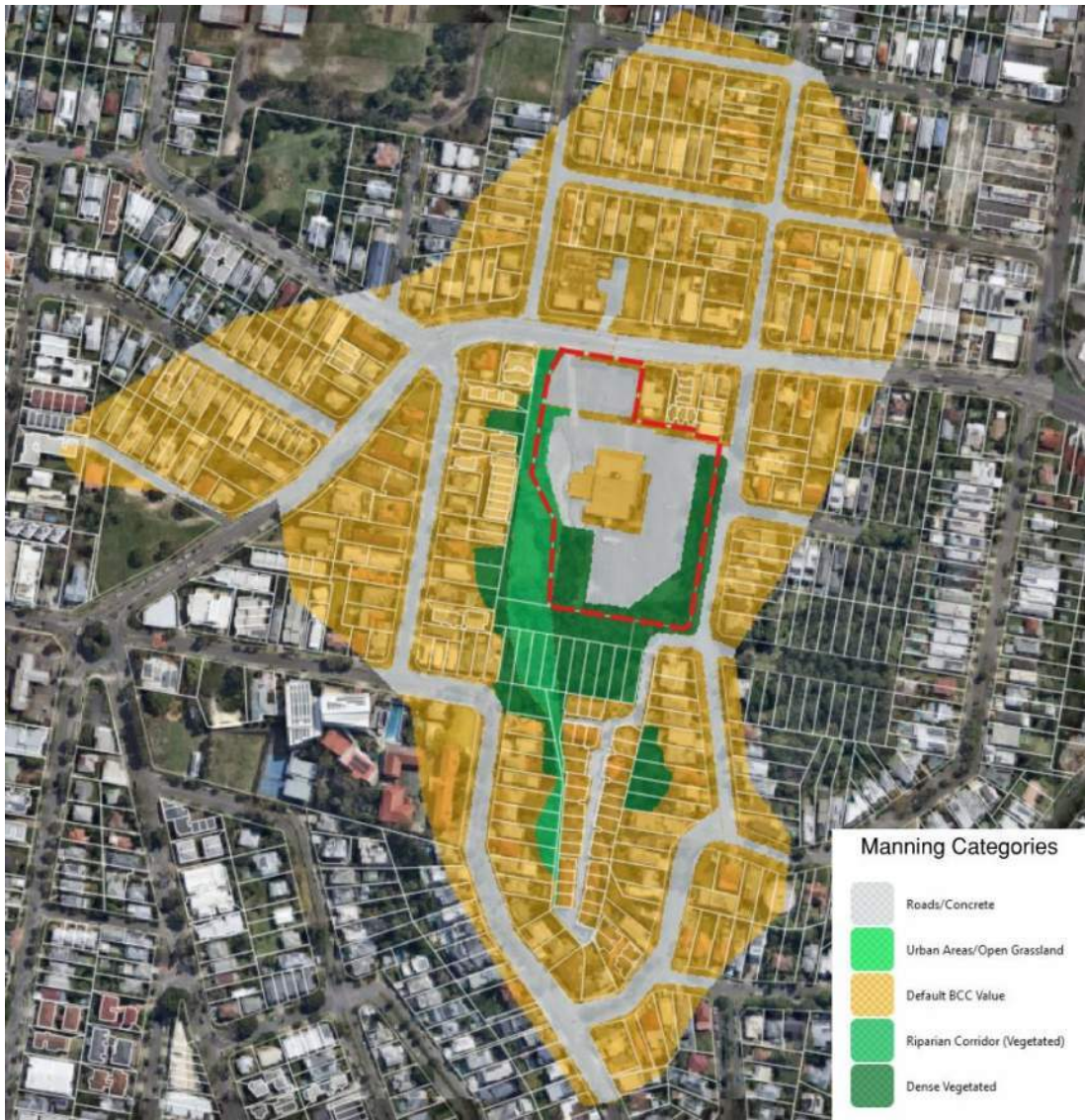
Figure 10 – Pre-Development Manning's n Roughness Mapping
