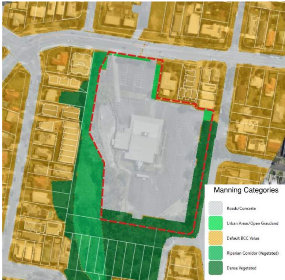
Figure 11 – Post-Development Manning's n Roughness Mapping
