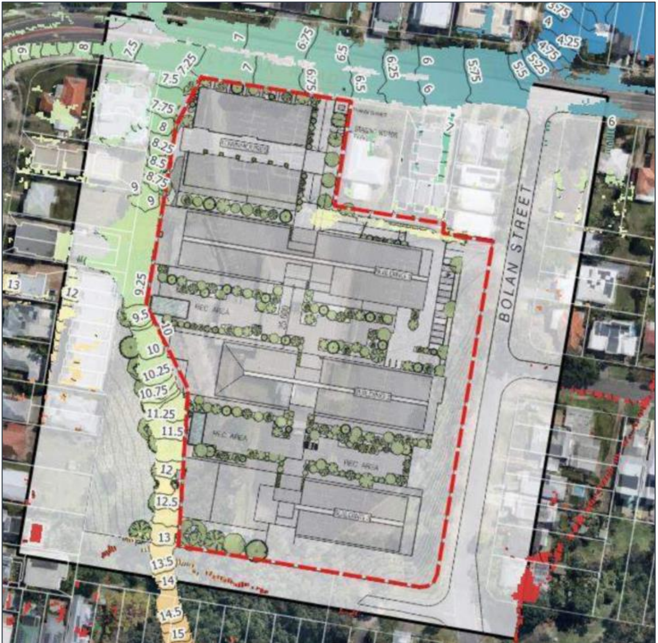
Figure 1. 2% AEP Overland Flow Flood Surface Levels (Courtesy: MPN)
